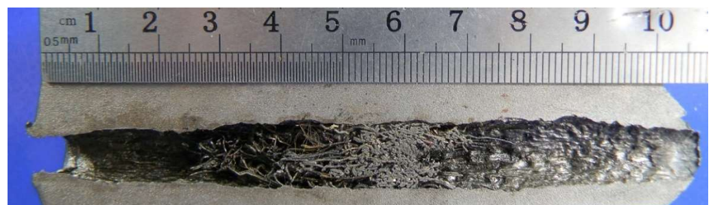
Figure 14. Longitudinal section of crater penetrated by the Ø5.6 mm WF(0.3)/Zr-MG rod.
