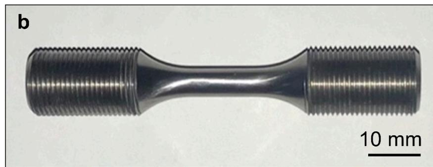
**Figure 2.** The schematic illustration (a) and macrograph (b) of specimens for the strain-controlled fatigue test (unit: mm).
