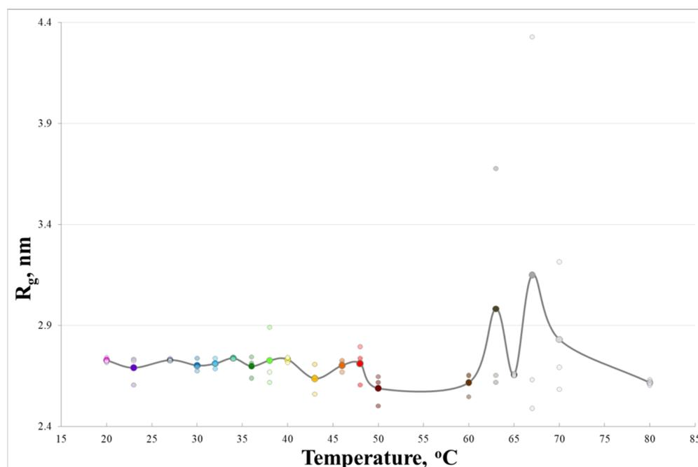
**Figure 6.**  $R_g$  of proteinase K dimers averaged over  $C_\alpha$  atoms at different temperatures (from 20 to 80 °C). Saturated connected points represent data averaged over three independent simulations marked by unsaturated points.
