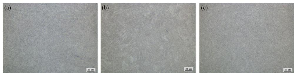
**Figure 8.** Microstructure of the welded joint of 155 mm-thick plates: (a) WZ; (b) CG-HAZ; (c) FG-HAZ.
