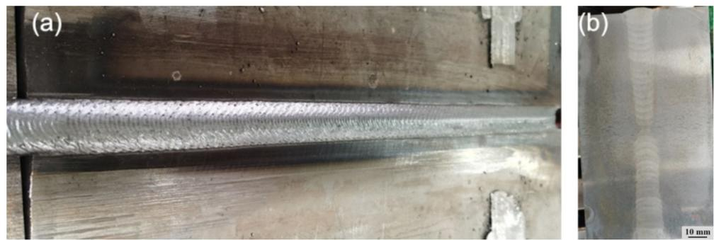
**Figure 7.** Weld appearance and cross-section of 135 mm-thick welded joint: (a) weld appearance; (b) cross-section.
