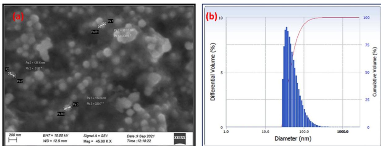
**Figure 5.** (a) Morphological appearance of phyto-synthesized MA-CNPs through SEM analysis. (b) DLS analysis of green synthesized MA-CNPs.
