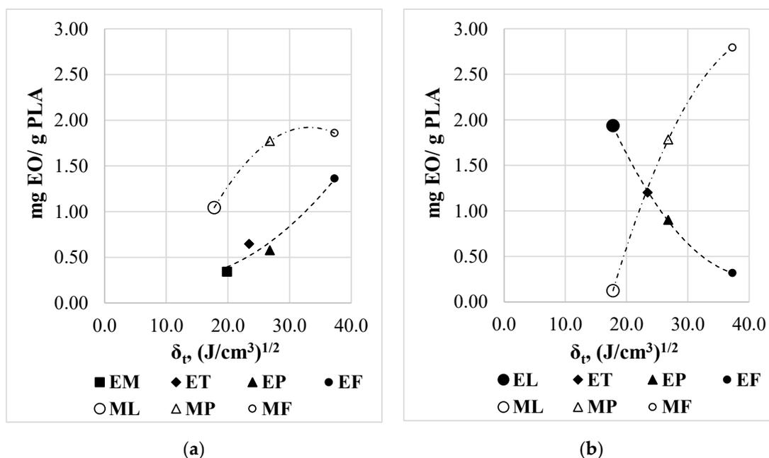
**Figure 8.** The specific amount of essential oil adsorbed as a function of the solubility parameter of essential oils in the case of sample *F* in: (a) 1.5 wt.% solutions, (b) 2 wt.% solutions with ethanol and methanol as a solvent.
