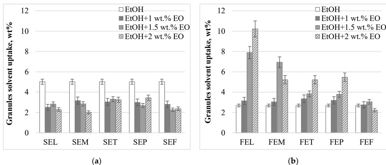
**Figure 1.** Solvent uptake in ethanol at different concentration of essential oil: (a) 4043D granules; (b) 3D850 granules.
