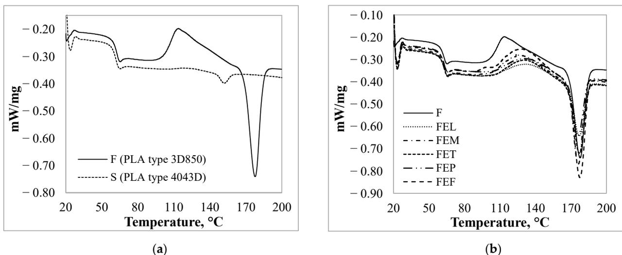
**Figure 9.** DSC thermograms of the samples: (a) DSC curves of the two PLA granules, (b) DSC curves of 3D850 PLA granules after adsorption.
