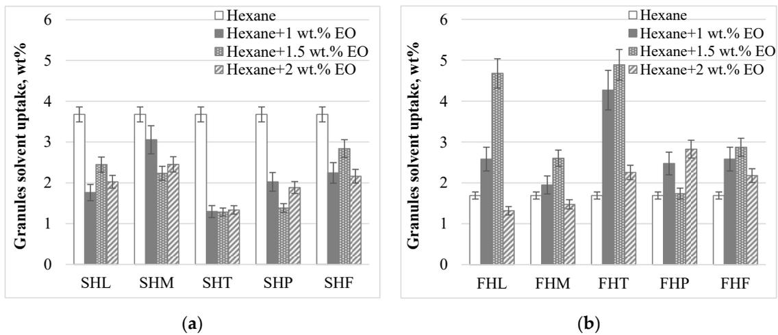
**Figure 3.** Solvent uptake in hexane at different concentration of essential oil: (a) 4043D granules; (b) 3D850 granules.
