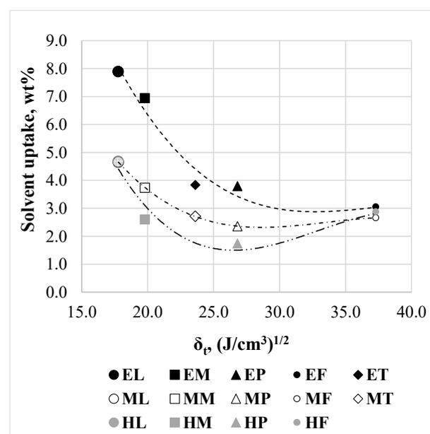
**Figure 7.** Solvent uptake as a function of the solubility parameter of essential oils in the case of 1.5 wt.% solution concentration with ethanol, methanol and hexane solvent.
