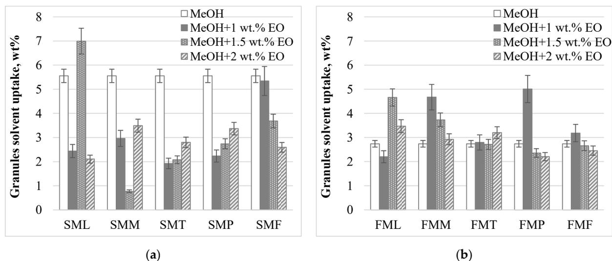
**Figure 2.** Solvent uptake in methanol at different concentration of essential oil: (a) 4043D granules; (b) 3D850 granules.
