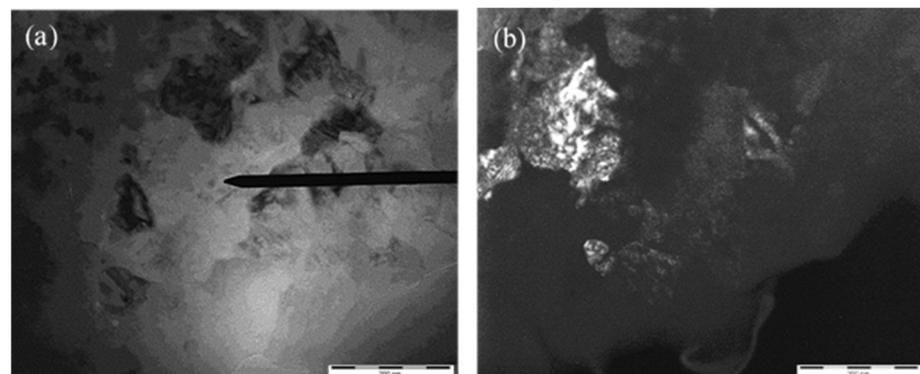
**Figure 7.** Electron microscopic images of the thin structure of detonation coating based on  $\text{Ti}_3\text{SiC}_2$  before and after pulse-plasma treatment: (a)—brightfield image before the PPT, (b)—darkfield image after the PPT.
