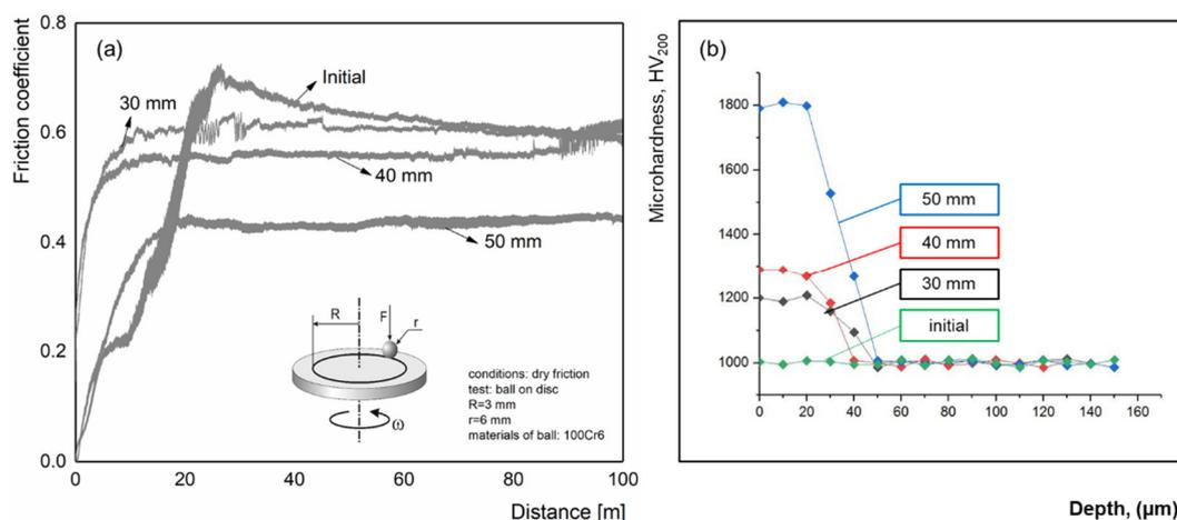
**Figure 10.** Results of tribological studies (a) and microhardness on the cross-section of the coatings (b).
