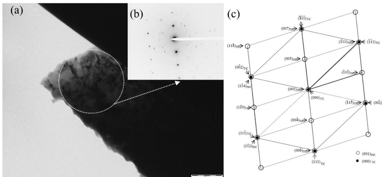
**Figure 9.** TEM images of the substructure of detonation coating based on  $\text{Ti}_3\text{SiC}_2$  after pulse-plasma treatment: (a)—brightfield image of the thin structure of  $\text{Ti}_3\text{SiC}_2$ ; (b)—microdiffraction pattern obtained of the selected area on (a); (c)—indexed diagram.
