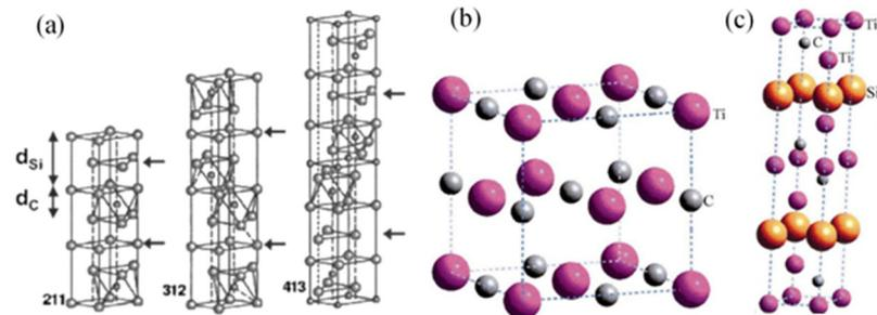
**Figure 6.** Crystal structure of MAX phases from different sources: (a)  $M_{n+1}AX_n$  phase structures for  $n = 1, 2$  and  $3$  [28]; (b) TiC crystal structure [26]; (c)  $\text{Ti}_3\text{SiC}_2$  crystal structure [26].
