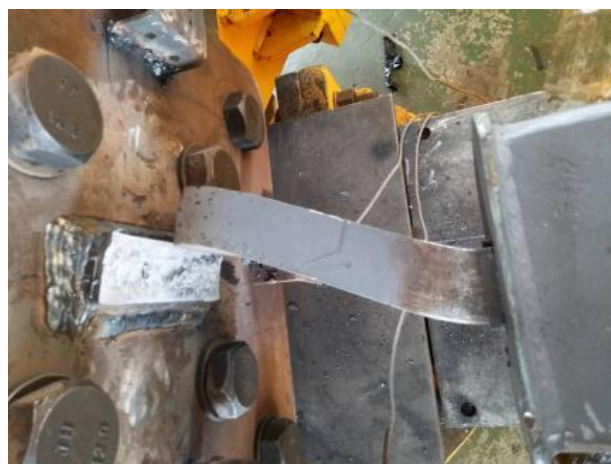
Figure 3. Out-of-plane deflection of the stiffening part.
