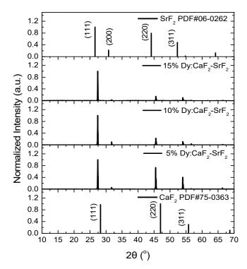
Figure 2. XRD pattern of Dy:CaF<sub>2</sub>-SrF<sub>2</sub> crystal.
