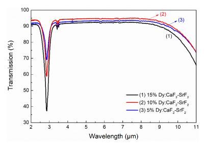
**Figure 3.** Transmission spectra of Dy:CaF<sub>2</sub>-SrF<sub>2</sub> crystals at 2–11 μm.
