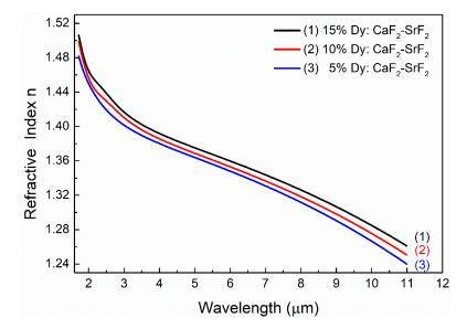
Figure 4. Refractive index of Dy:CaF<sub>2</sub>-SrF<sub>2</sub> in the mid-IR spectral range of 1.7–11 μm.
