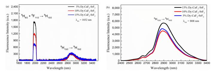
Figure 6. Emission spectra of Dy:CaF<sub>2</sub>-SrF<sub>2</sub> crystal under different pump source. (a) 1320 nm pump; (b) 808 nm pump.
