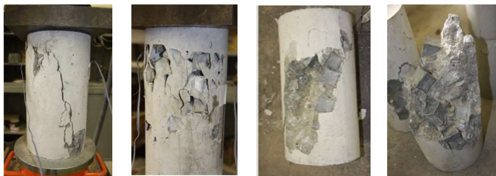
Figure 26. The failure mode of concrete specimens mixed with multiple concave bodies.
