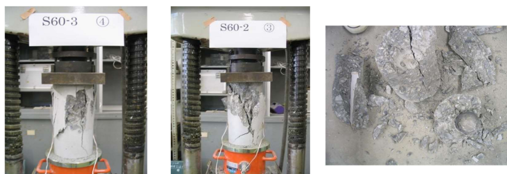
Figure 8. The failure mode of concrete specimens mixed with a single sphere.
