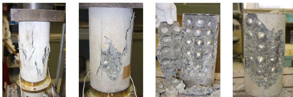
Figure 32. The failure mode of concrete specimens mixed with fixed sphere positions.
