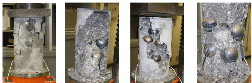
Figure 21. The failure mode of concrete specimens mixed with multiple spheres.
