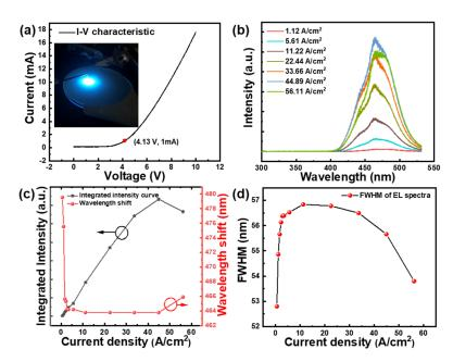
Figure 4. (a) The I-V characteristic of wafer-scale pyramid  $\mu$ LED array measured through on-wafer electrical probing; the inset is a photograph of the LED operated at 22.44 A/cm<sup>2</sup>; (b) EL spectra of the wafer-scale pyramid  $\mu$ LED array as a function of injected current density; (c) the integrated EL intensity and wavelength peak shift curve as a function of injected current density; (d) the FWHM of EL spectra as a function of injected current density.
