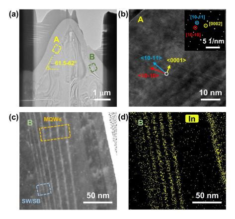
**Figure 3.** (a) TEM image of a single pyramid  $\mu$ LED structure; (b) HRTEM image of region A in (a), including part of the MQWs structure and the p-GaN layer; inset is the image of corresponding SAED patterns; (c) HAADF STEM image of region B in (a), including MQWs and p-GaN layer in the  $\mu$ LED structure; (d) EDS mapping of In element in MQWs, corresponding to (c).
