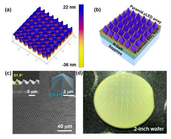
Figure 1. (a) AFM image of the as-fabricated patterned SiO<sub>2</sub> layer on n-GaN template; (b) Schematic diagram of the as-grown pyramid  $\mu$ LED array on patterned SiO<sub>2</sub> layer; (c) The 25° tilted SEM image (magnification: 500×) of the as-grown pyramid  $\mu$ LED array. The insets represent the cross-section SEM image and a magnified pyramid structure; (d) Photograph of the 2-inch wafer with pyramid  $\mu$ LED array.
