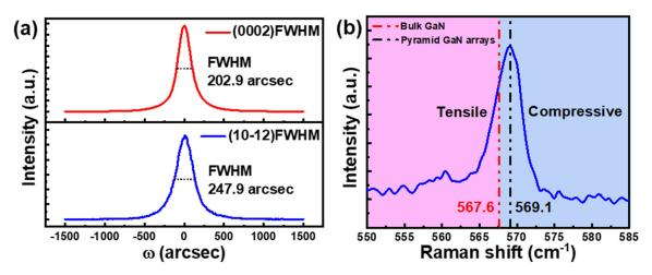
Figure 2. (a) XRD (0002) and (10-12) rocking curves, and (b) Raman spectrum of the as-grown pyramid  $\mu$ LED epitaxial structure on patterned SiO<sub>2</sub> layer.
