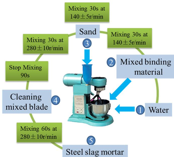
Figure 3. Mixing progress of steel slag mortar.
