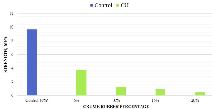
Figure 11. Compressive strength (after heating) at 28 days.
