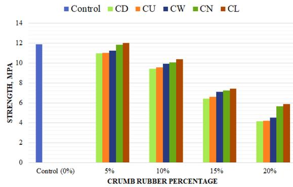
Figure 8. Compressive strength at 7 days.
