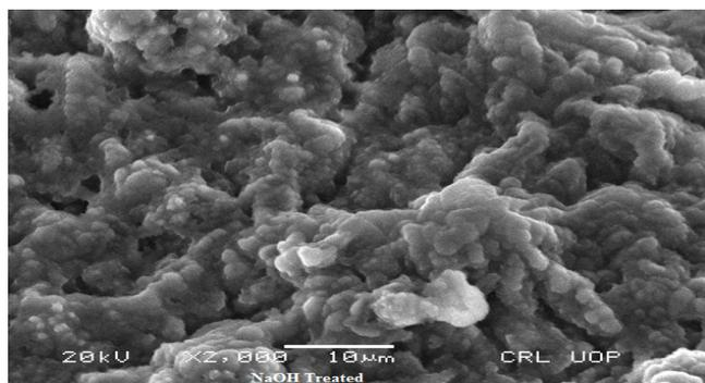
Figure 17. NaOH-treated CR.
