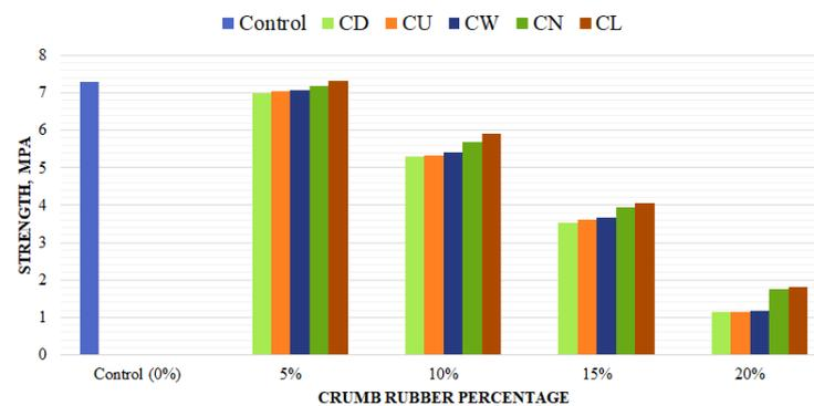
Figure 12. Indirect tensile strength at 28 days.
