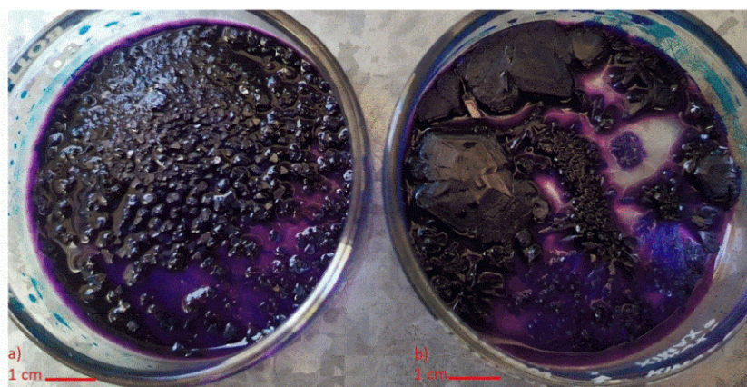
Figure 4. (a) crystals without UV assistance; (b) crystals with UV assistance.
