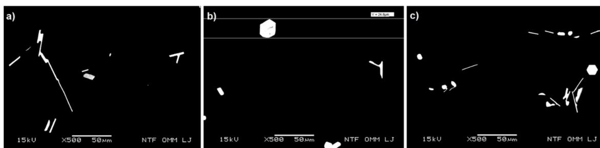
**Figure 6.** Plate, angular, and hexagonal  $Mg_3Bi_2$  phases (bright areas) (a) 1M150, (b) 2M150 (c) 3M105 (BEI-higher magnification).
