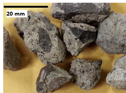
Figure 23. A low magnification image showing adhered cement in a RAC [168]. Reprinted with permission from Elsevier [168].
