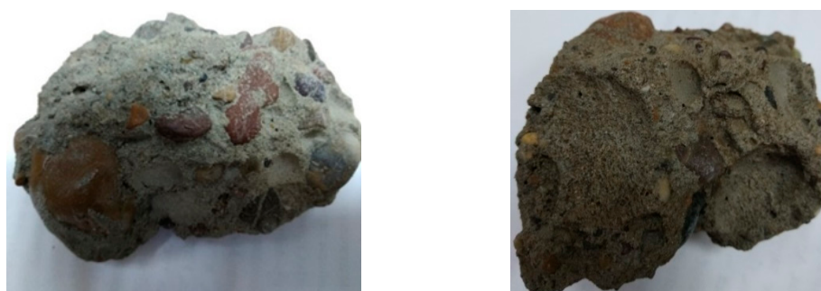
Figure 2. Original rough surfaces of the RCAs.
