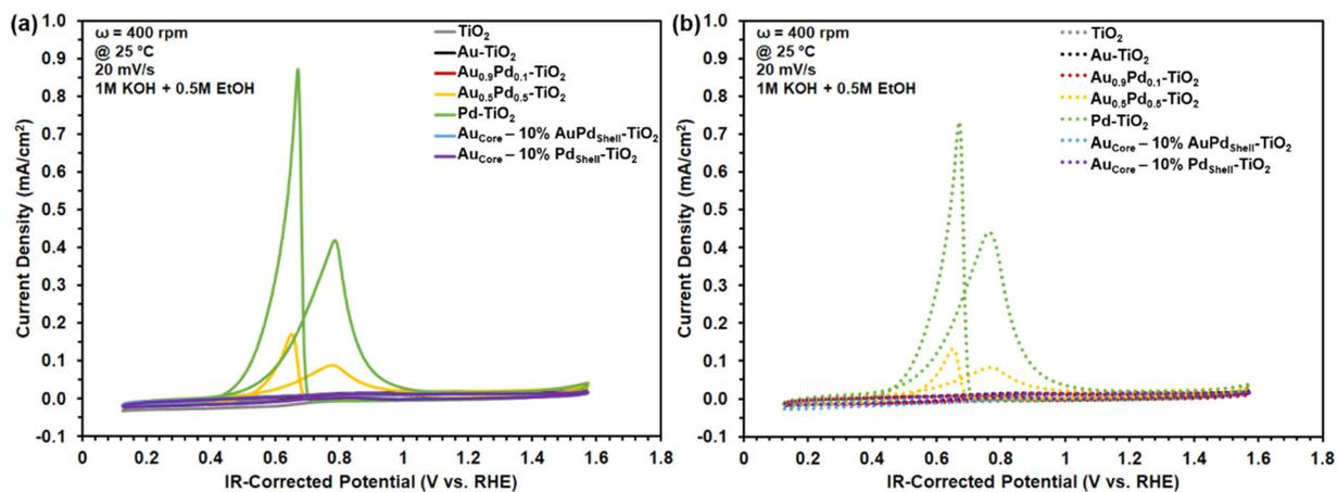
**Figure S11.** Electrochemical CVs of EtOH oxidation catalyzed by 1 wt% Au<sub>1-x</sub>Pd<sub>x</sub> and Au<sub>Core</sub>-Au<sub>1-x</sub>Pd<sub>x</sub>.Shell NPs dispersed on TiO<sub>2</sub> deposited onto a rotating disk, glassy carbon working electrode immersed into 0.5 M EtOH with 1 M KOH supporting electrolyte. Reference and counter electrodes were Ag/AgCl and a Pt coil, respectively. CVs of the current density in the (a) dark and under (b) AM1.5G irradiation.
