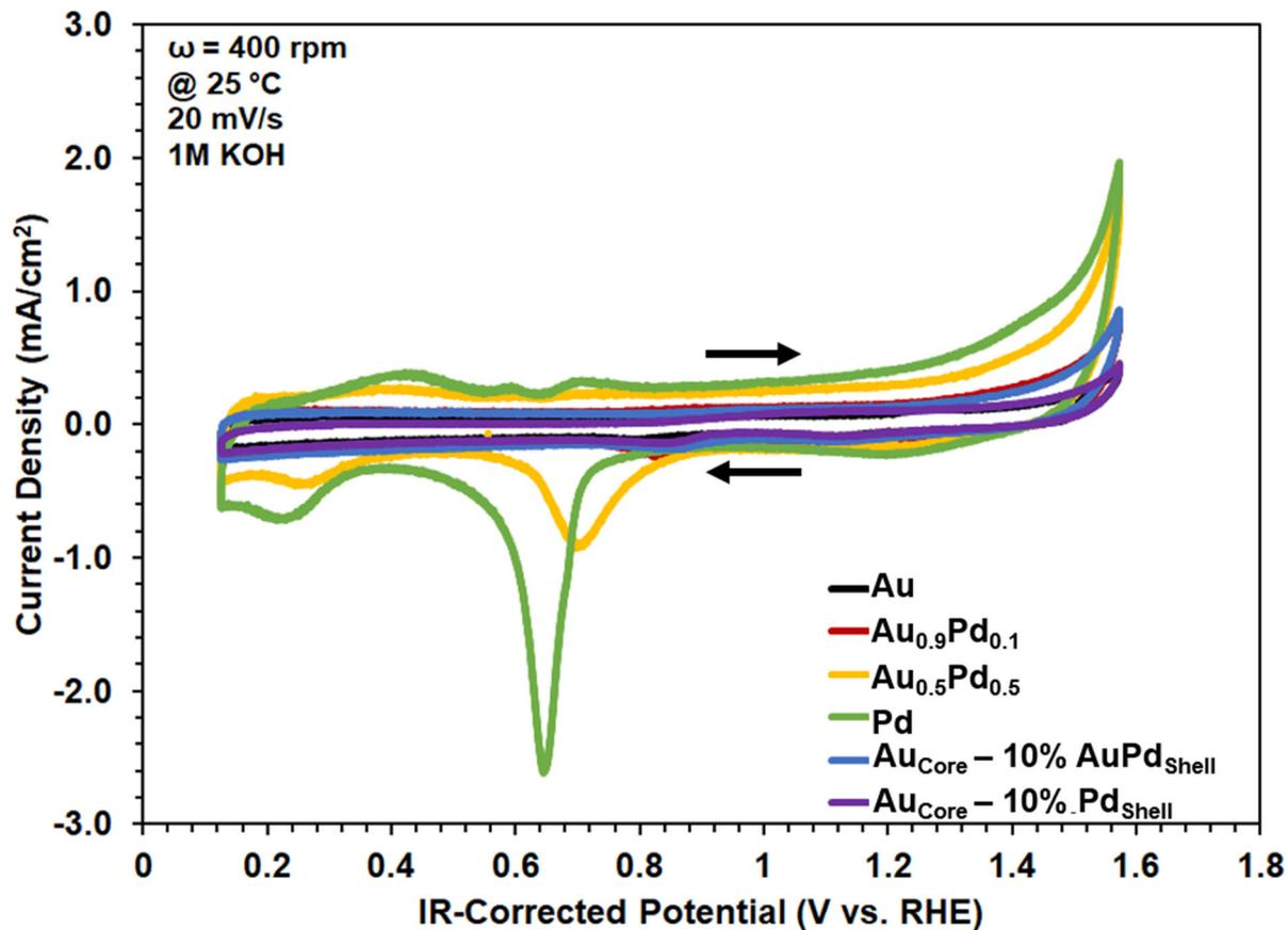
**Figure S9.** Electrochemical CVs in 1 M KOH supporting electrolyte (pH~14) catalysed by 60  $\mu\text{g}$  of 20 wt%  $\text{Au}_{1-x}\text{Pd}_x$  and  $\text{Au}_{\text{Core}}\text{-Au}_{1-x}\text{Pd}_x\text{Shell}$  NPs dispersed on carbon supports deposited onto a rotating disk, glassy carbon working electrode in the dark. Reference and counter electrodes were Ag/AgCl and a Pt coil, respectively.
