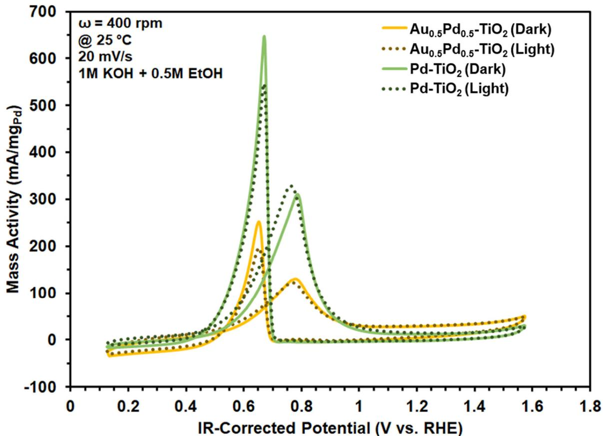
**Figure S12.** Electrochemical CVs of EtOH oxidation catalyzed by 1 wt% AuPd and Pd NPs dispersed on TiO<sub>2</sub> deposited onto a rotating disk, glassy carbon working electrode immersed into 0.5 M EtOH with 1 M KOH supporting electrolyte. Reference and counter electrodes were Ag/AgCl and a Pt coil, respectively. CVs of the mass activity (Pd) in the dark and under AM1.5G irradiation.
