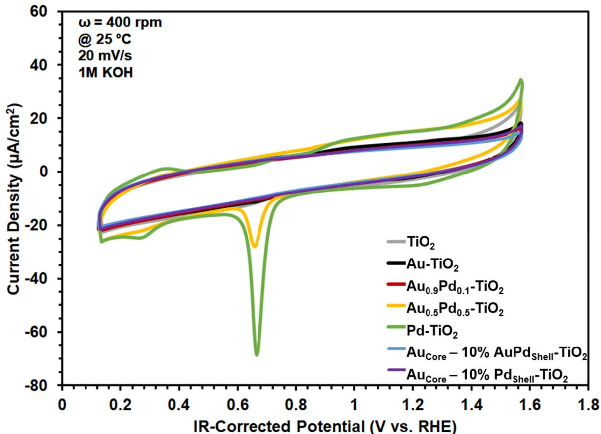
**Figure S10.** Electrochemical CVs in 1 M KOH supporting electrolyte (pH~14) catalysed by 60  $\mu\text{g}$  of 1 wt%  $\text{Au}_{1-x}\text{Pd}_x$  and  $\text{Au}_{\text{Core}}\text{-Au}_{1-x}\text{Pd}_x\text{.Shell}$  NPs dispersed on  $\text{TiO}_2$  supports deposited onto a rotating disk, glassy carbon working electrode in the dark. Reference and counter electrodes were Ag/AgCl and a Pt coil, respectively.
