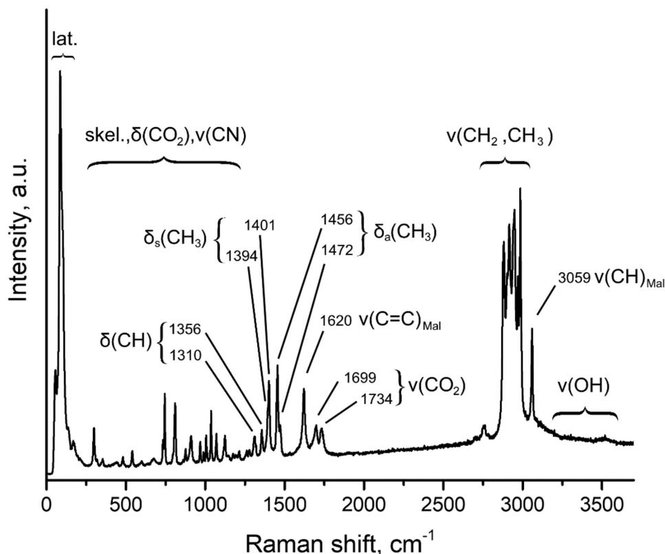
**Figure 3.** Experimental Raman spectra bands assignment in LLHM crystal structure at 298 K. Calculated gas-phase vibrational spectra are presented in Figure S1 (please see Supplementary Materials).
