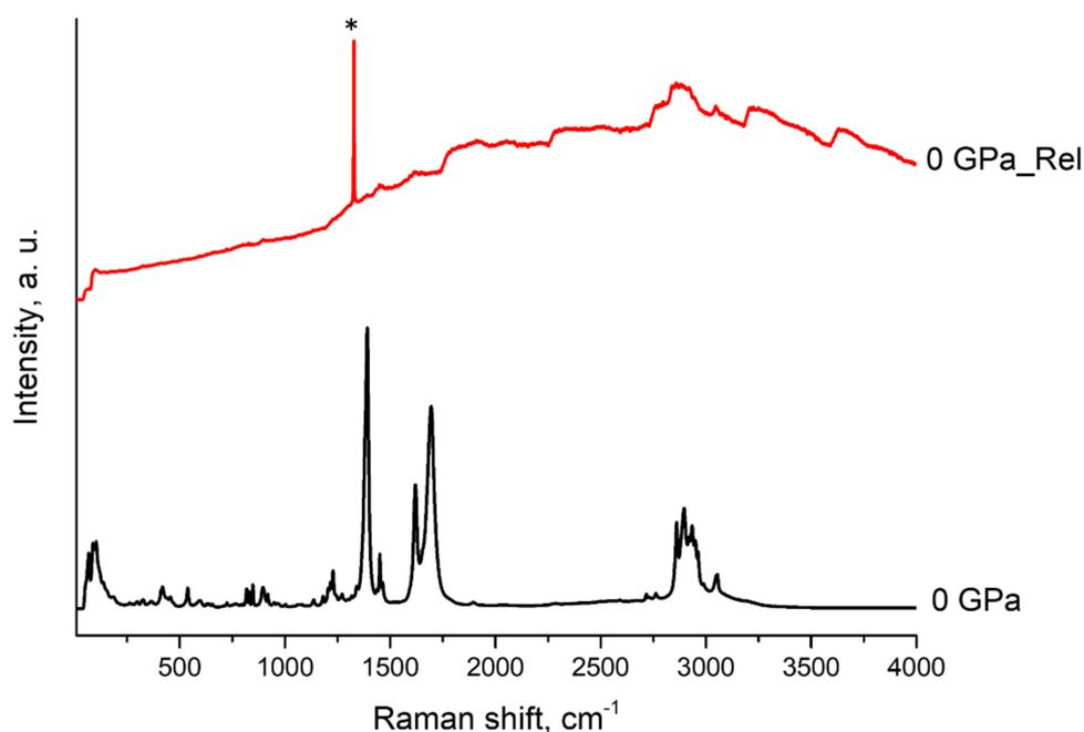
**Figure 6.** Raman spectra of LLHM at PIP PTM at 0 GPa before (bottom black line) and after (upper red line) pressure impact. \* Asterisk mark the signal from DAC.
