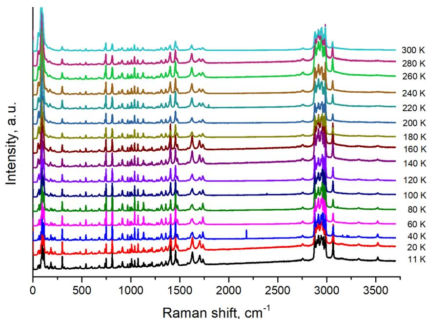
**Figure 4.** LLHM Raman spectra at low temperatures, showing no phase transition on cooling. Lone spurious peaks in the region of 2000–2500  $\text{cm}^{-1}$  at temperatures 40 and 100 K were not vanished from spectra to preserve original data. Same is true for spurious peaks at 40 K in the region between 3100–3250  $\text{cm}^{-1}$ .
