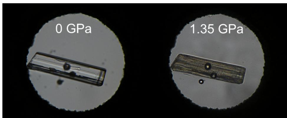
**Figure 7.** Photographs showing LLHM crystal destruction in PIP at pressure 1.35 GPa. LLHM crystal at 0 GPa (left) and 1.35 GPa (right). Crystal size is 0.3 mm × 0.05 mm × 0.02 mm.
