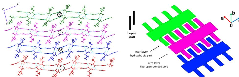
**Figure 1.** Crystallographic (left) and schematic (right) representation of the layered structure of LLHM, showing layers that shift resulting in plasticity under mechanical stress (adapted from [34,35]). Layers’ shifts are marked with an arrow sign depending on the direction of displacement.
