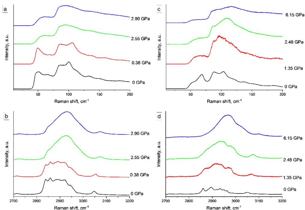
**Figure 5.** Raman spectra of LLHM at multiple pressures at (a,c) low-frequency and (b,d) high-frequency regions, showing different behavior in paraffin (left) and PIP (right) PTM.
