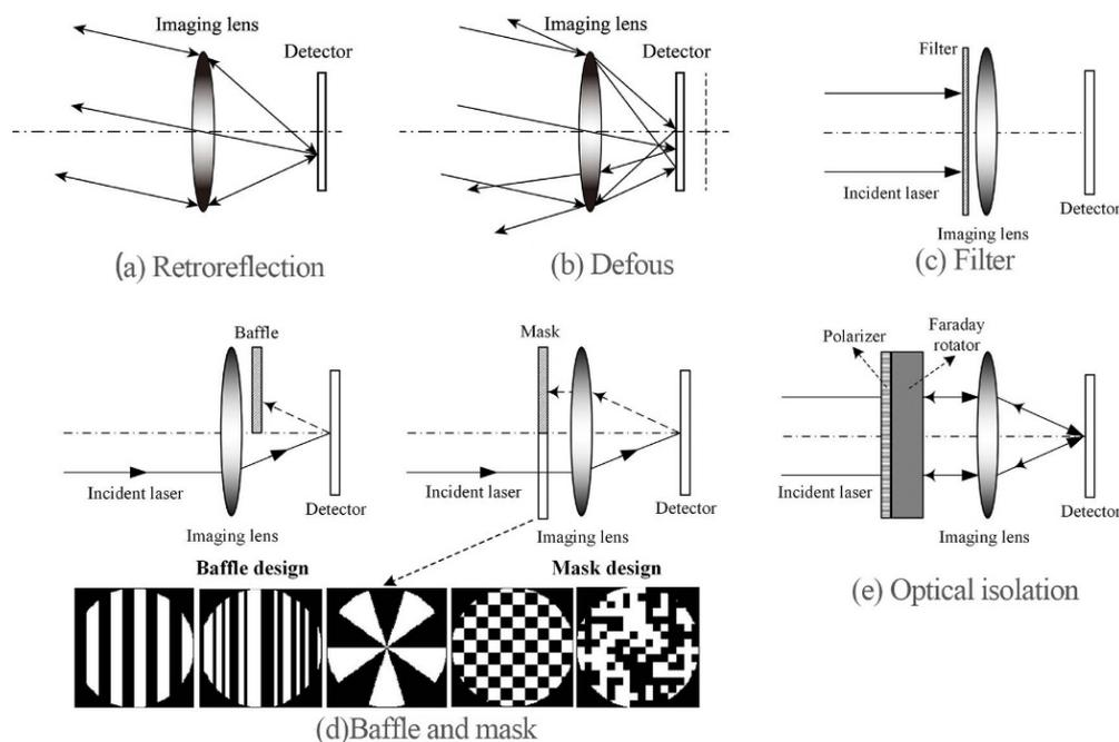
**Figure 1.** (a) The principle of retroreflection effect and (b–e) a few methods to reduce the strength of the retroreflected signal.
