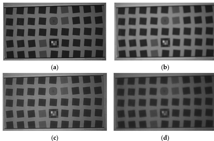
**Figure 5.** Experimental results of conventional imaging system and wavefront coding imaging system under defocus conditions, (a) image of conventional imaging system in focusing state; (b) decoded image of conventional imaging system under 10 units defocus amounts; (c) image of wavefront coding system in focusing state; (d) decoded image of wavefront coding system in 10 units positive defocusing state.
