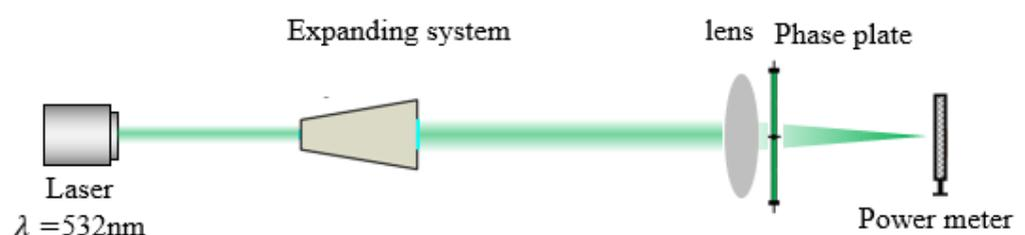
**Figure 8.** Sketch map of the experimental setup to measure the transmittance of phase plate.
