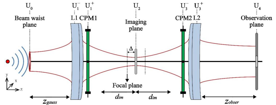
Figure 2. Equivalent physical model of retroreflection in wavefront coding imaging system.
