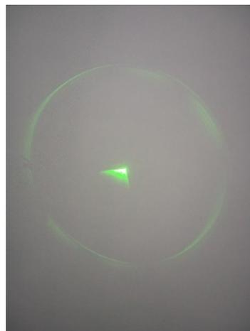
**Figure 7.** Far-field diffraction spot of the wavefront coded imaging system.
