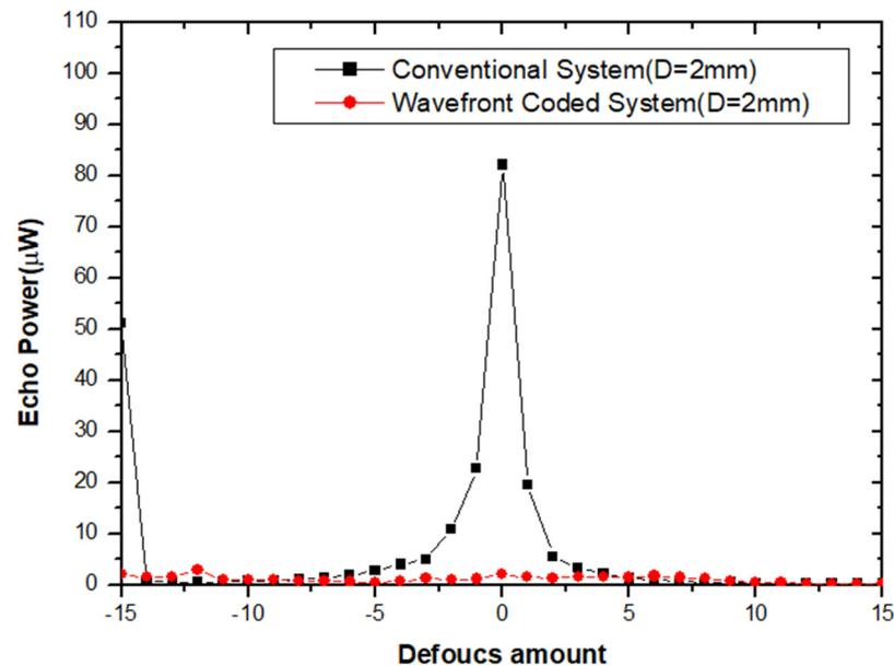
**Figure 9.** Comparison of the power of cat-eye echo in conventional and wavefront coded imaging system.
