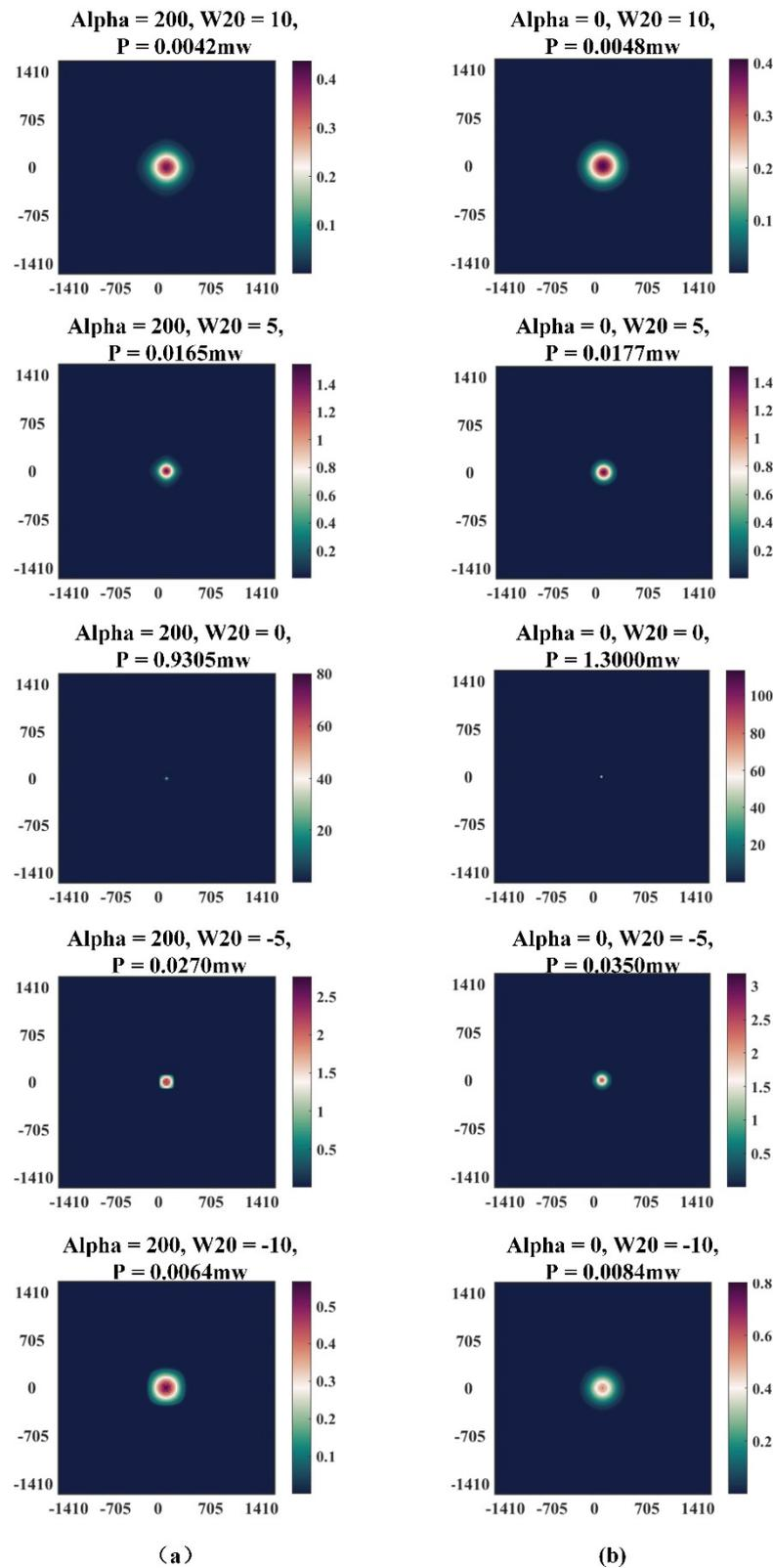
**Figure 4.** The cat-eye echo at a 20 m distance of (a) the conventional imaging system and (b) wavefront coded imaging system along with the corresponding echo-detector receiving power.
