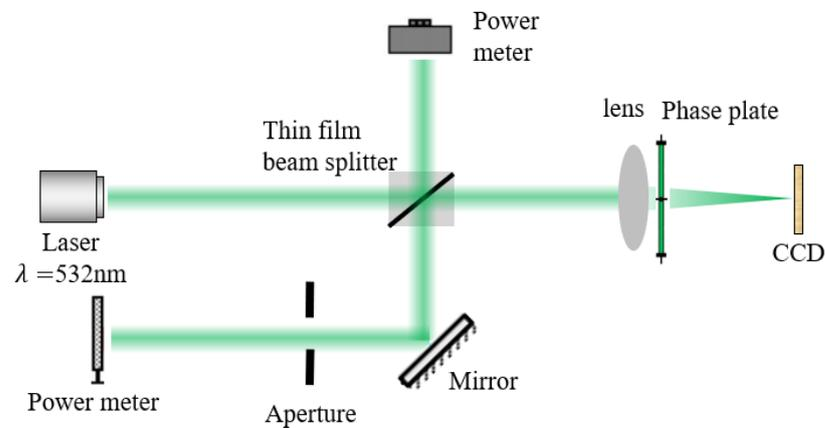
**Figure 6.** Sketch map of the experimental setup for a laser beam through a cat-eye system.
