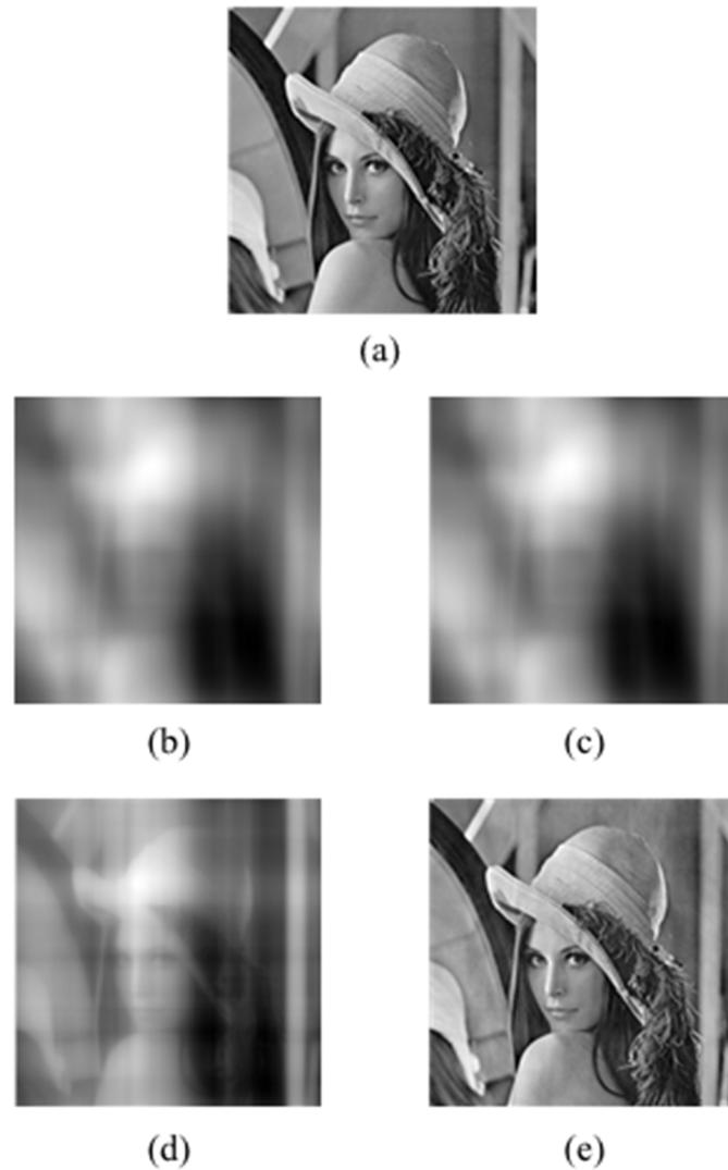
**Figure 3.** Comparison of imaging quality between conventional imaging system and wavefront coding imaging system under different defocus amounts. (a) original image; (b) intermediate coded image obtained by conventional imaging system under a defocus amount of 10 units; (c) decoded image from conventional imaging system; (d) intermediate coded image obtained by wavefront coding system under a defocus amount of 10 units; (e) decoded image from wavefront coding system.
