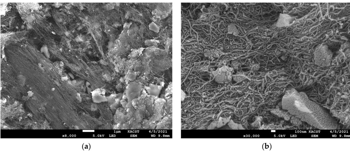
Figure 6. SEM images of 0.75 wt% MWCNT and silica gel composite at (a) 1 μm and (b) 100 nm scale.
