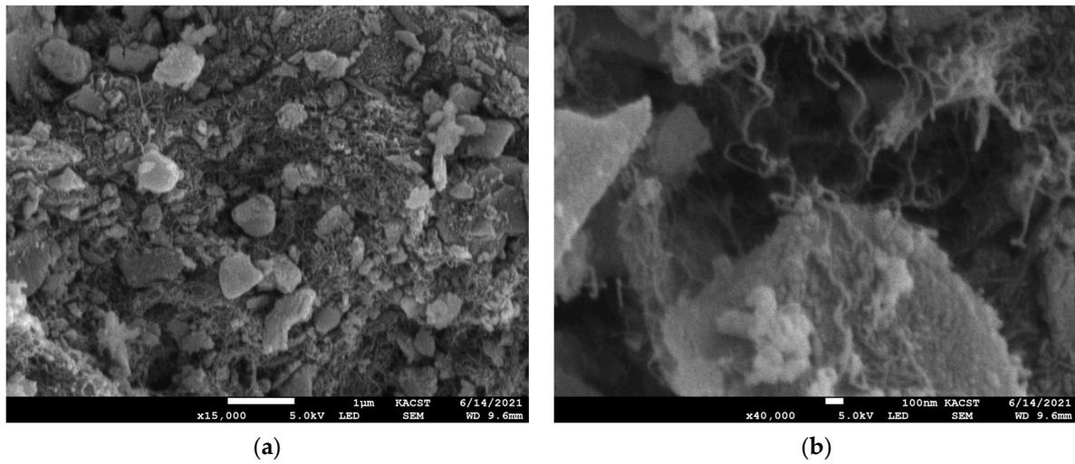
Figure 4. SEM images of 0.25 wt% MWCNT and silica gel composite at (a) 1 μm and (b) 100 nm scale.
