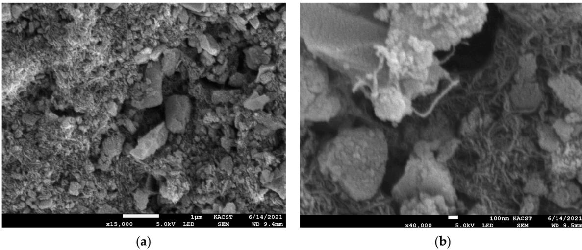
Figure 5. SEM images of 0.5 wt% MWCNT and silica gel composite at (a) 1 μm and (b) 100 nm scale.
