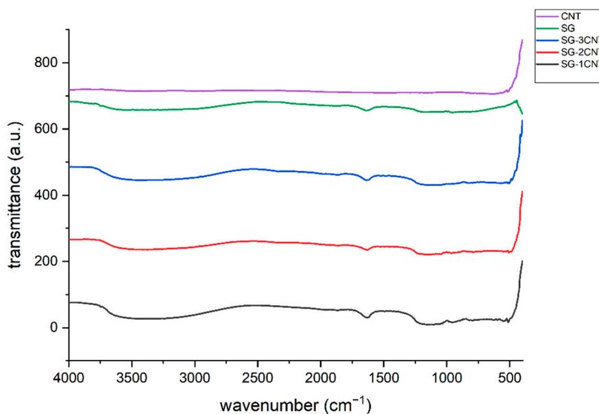
**Figure 7.** Results of FTIR test for MWCNTs, silica gel composites, and SG/xMWCNTs ( $x = 0.25, 0.50$ , and  $0.75\text{ wt}\%$ ).
