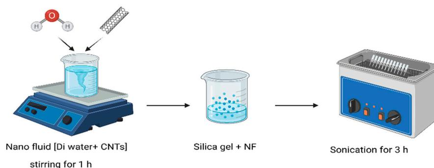
**Figure 1.** Preparation procedure for silica gel with MWCNTs.
