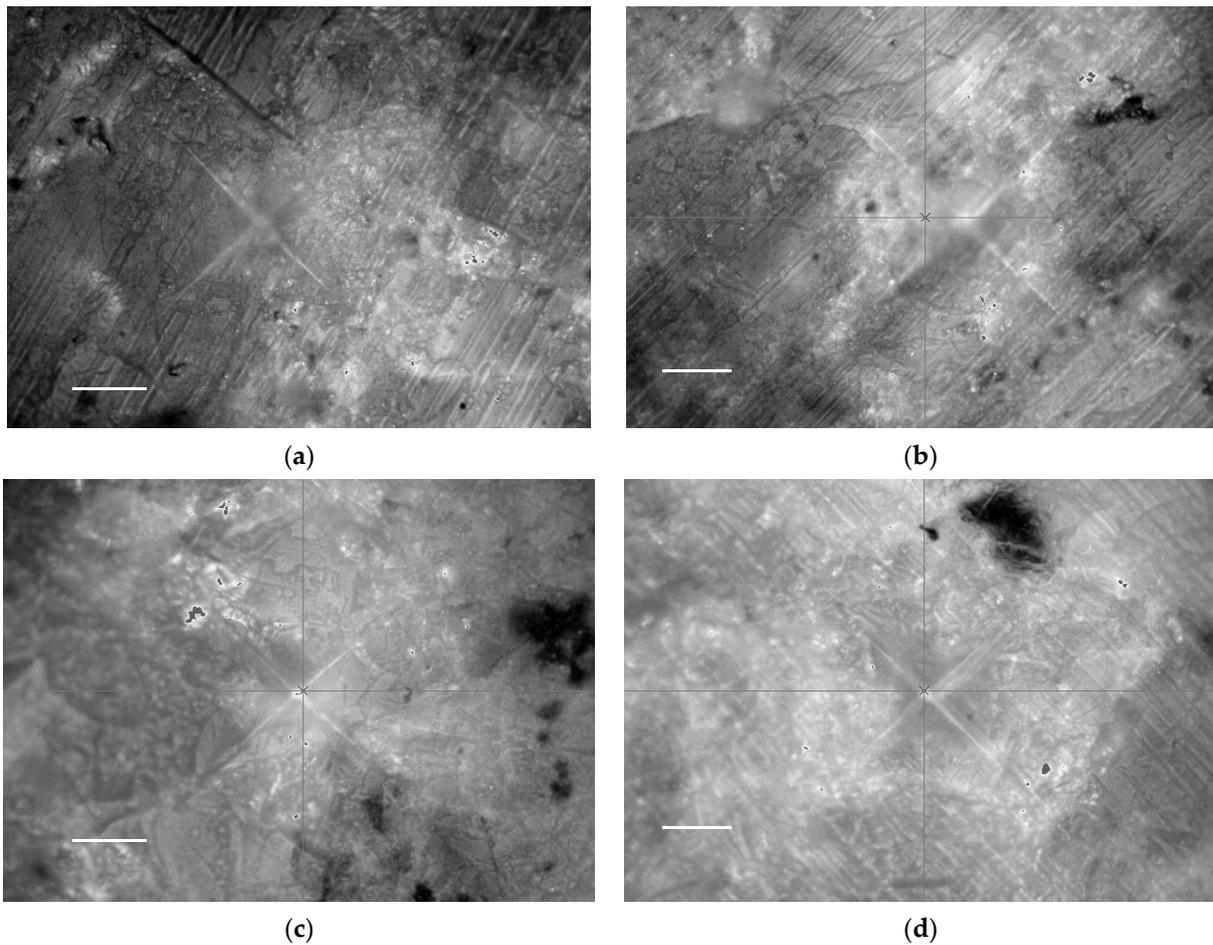
**Figure 11.** Optical micrographs of Vickers residual indentations of silica gel and MWCNT composites at 300 K: (a) SG . CNT silica gel at (b) 0.25 wt%, (c) 0.5 wt%, and (d) 0.75 wt%. Edges of indentation along with diagonal cracks are clearly defined. See scale bar is a 100  $\mu\text{m}$ .
