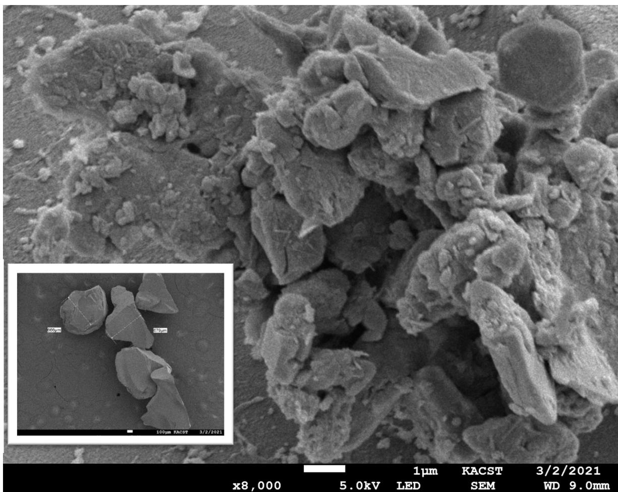
**Figure 3.** SEM image of silica gel particles; image scale bar indicates 1  $\mu\text{m}$ . The inset image shows that their average size is above 500  $\mu\text{m}$ .
