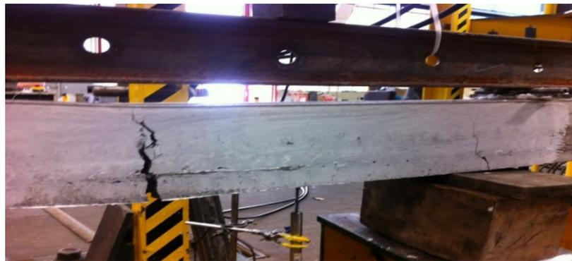
**Figure 9.** The failure mode and cracks pattern of BT<sub>(5cm)14</sub>-Anch-2.6-L, 50k TRC beam.
