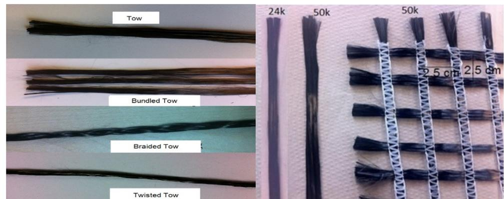
**Figure 1.** Multi-filament carbon fibres used as reinforcement of TRC beams.
