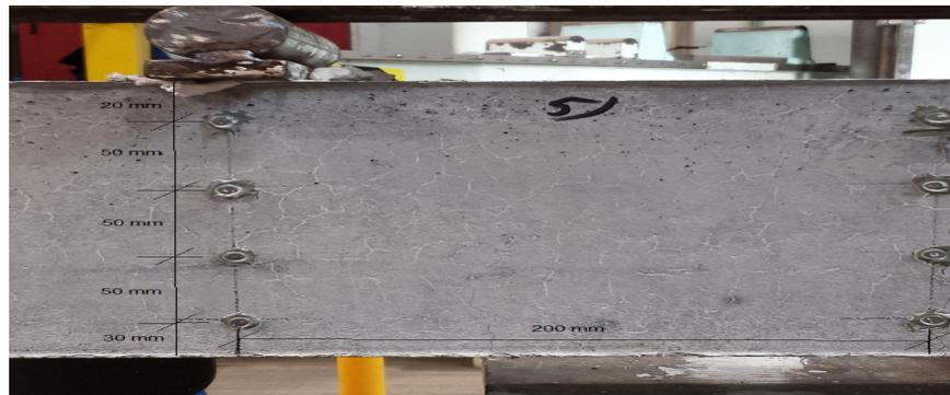
Figure 3. The arrangement of demecs on the surface of beams.
