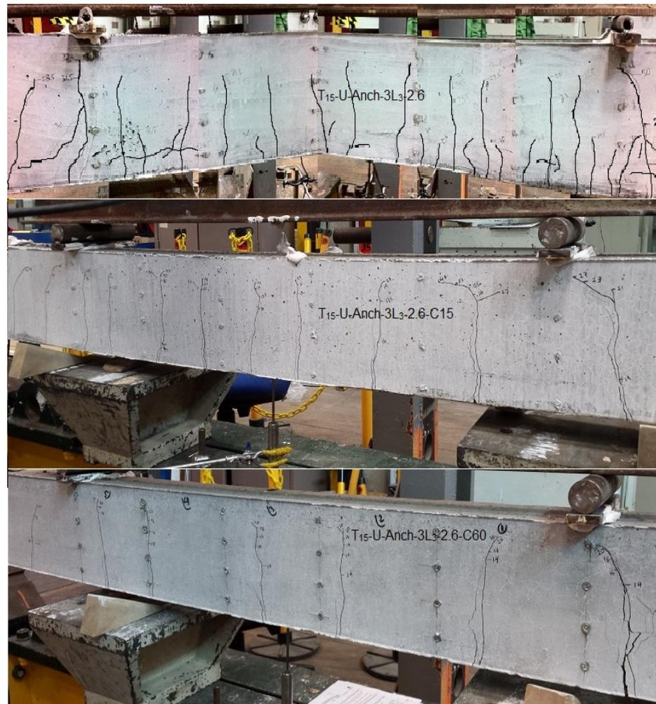
**Figure 22.** The failure modes and crack patterns of TRC beams with various covers.
