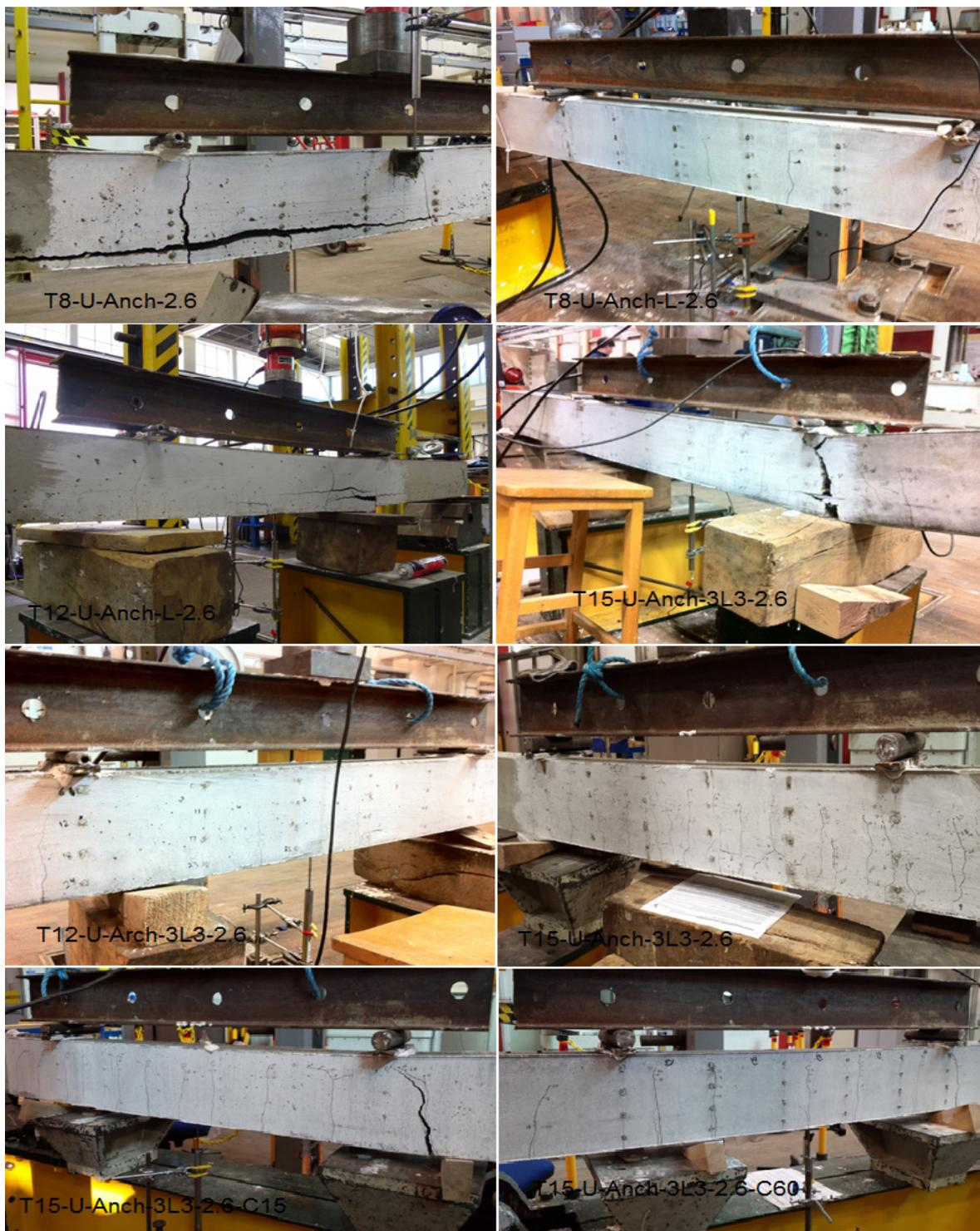
Figure 13. The mods of failure and crack patterns of uni-axial TRC beams.
