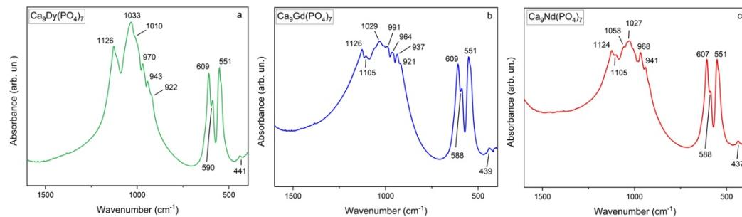
**Figure 7.** FTIR spectra of (a)  $\text{Ca}_9\text{Dy}(\text{PO}_4)_7$ , (b)  $\text{Ca}_9\text{Gd}(\text{PO}_4)_7$ , and (c)  $\text{Ca}_9\text{Nd}(\text{PO}_4)_7$  in the  $1600\text{--}400\text{ cm}^{-1}$  region.
