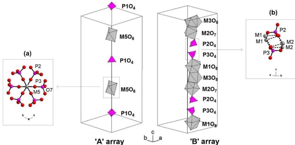
**Figure 5.**  $\text{Ca}_9\text{RE}(\text{PO}_4)_7$  packing: A and B arrays. Inset (a): detail of  $[\text{M}_5(\text{PO}_4)_6]$  unit. Inset (b): joining mechanism among B arrays (M-O bonds dashed).
