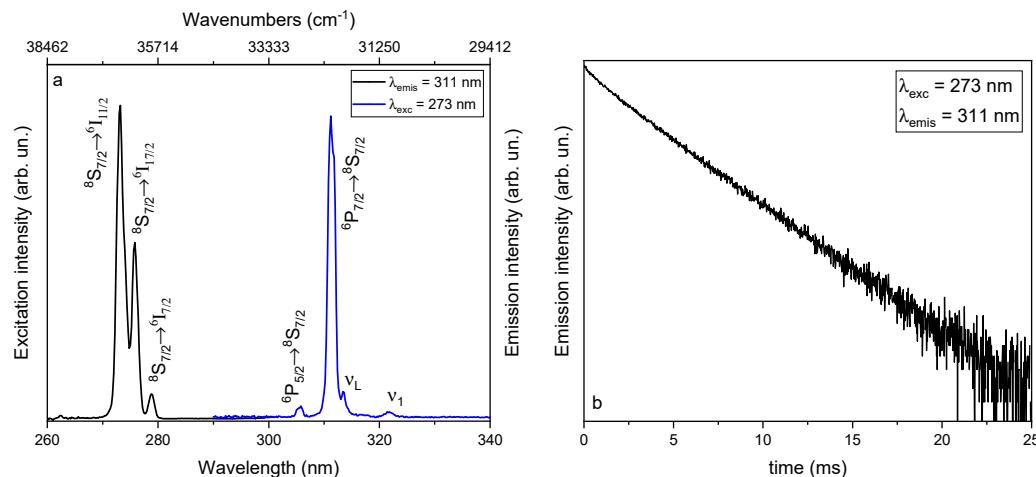
**Figure 10.** (a) Excitation spectrum of Ca<sub>9</sub>Gd(PO<sub>4</sub>)<sub>7</sub> (black line) at  $\lambda_{\text{emis}} = 311$  nm. Emission spectrum of Ca<sub>9</sub>Gd(PO<sub>4</sub>)<sub>7</sub> (blue line) at  $\lambda_{\text{exc}} = 273$  nm. (b) Decay time obtained for the compound Ca<sub>9</sub>Gd(PO<sub>4</sub>)<sub>7</sub> upon excitation at 273 nm and by detecting the emission at 311 nm.
