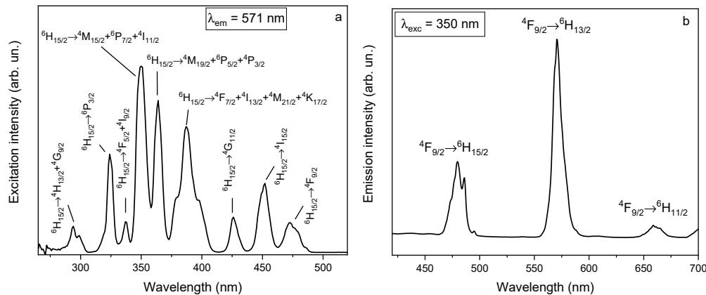
**Figure 8.** Excitation (a) and emission (b) spectra of  $\text{Ca}_9\text{Dy}(\text{PO}_4)_7$ .
