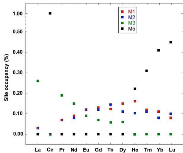
**Figure 4.** Distribution of *RE* cations within M1, M2, M3, and M5 sites in available  $\text{Ca}_9\text{RE}(\text{PO}_4)_7$  structure refinements; data from [6], with the exception of Ce [30], Tb and Ho [32], and Lu [31].
