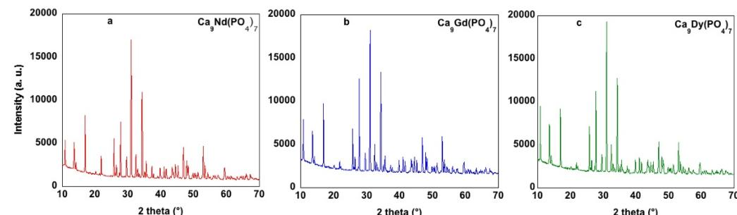
**Figure 1.** Powder X-ray spectra of  $\text{Ca}_9\text{Nd}(\text{PO}_4)_7$  (a),  $\text{Ca}_9\text{Gd}(\text{PO}_4)_7$  (b), and  $\text{Ca}_9\text{Dy}(\text{PO}_4)_7$  (c).
