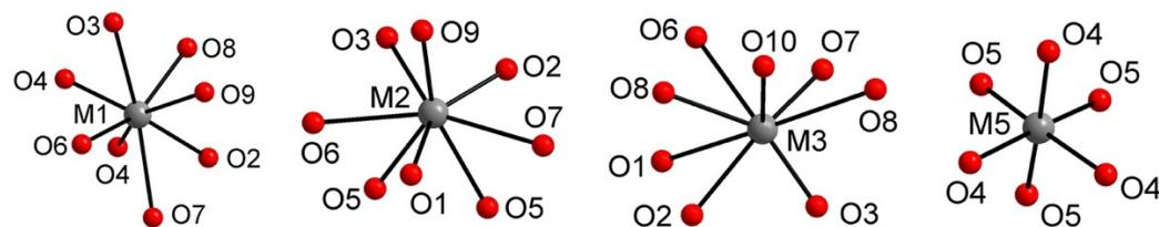
**Figure 3.** Polyhedral environment in structural sites of  $Ca_9RE^{3+}(PO_4)_7$   $\beta$ -TCP.
