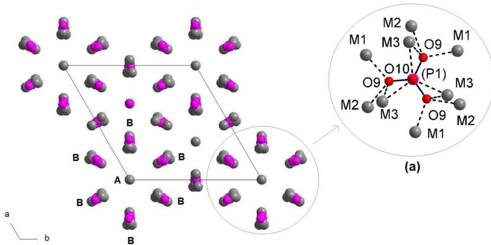
**Figure 6.** View down  $c$  of the  $\text{RE}$   $\beta$ -TCP framework. Inset (a):  $(\text{P}_1\text{O}_4)$  group environment and joining mechanisms with  $\text{M}_1\text{-}\text{M}_2\text{-}\text{M}_3$  polyhedra from adjacent B arrays.
