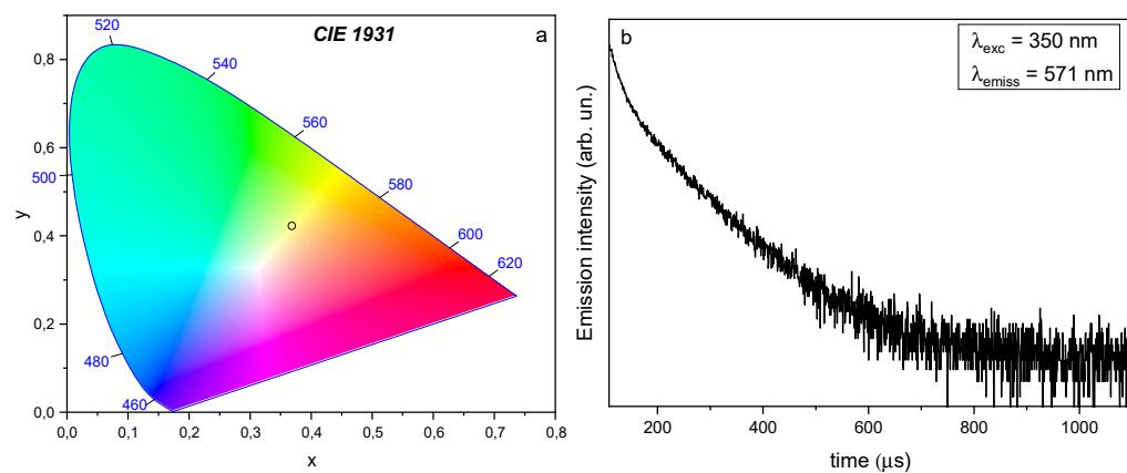
**Figure 9.** (a) CIE diagram for  $Ca_9Dy(PO_4)_7$  material upon excitation at 350 nm. (b) Decay time obtained for the compound  $Ca_9Dy(PO_4)_7$  upon excitation at 350 nm and by detecting the emission at 571 nm.
