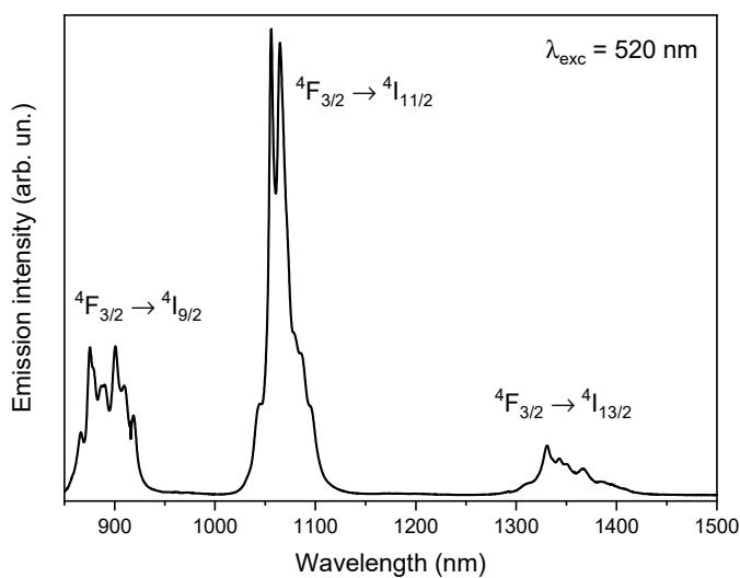
**Figure 11.** Emission spectrum of  $\text{Ca}_9\text{Nd}(\text{PO}_4)_7$  at  $\lambda_{\text{exc}} = 520 \text{ nm}$ .
