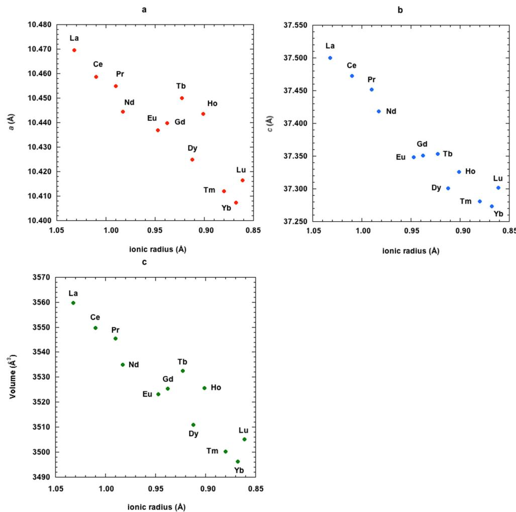
**Figure 2.** Unit cell parameters of  $\text{RE}$  β-TCP as a function of  $\text{RE}$  ionic radius (for 6-folded polyhedra). (a)  $a$  parameter (Å); (b)  $c$  parameter (Å); (c) Volume (Å<sup>3</sup>). Data from [6], except Ce [30], Lu [31], Tb and Ho [32].
