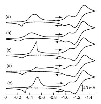
**Figure 11.** Cyclic voltammograms of (a)  $(Bu_4N)[Ni(dddt)_2]$ , (b) 1, (c) 2, (d) 3, and (e) 4. Conditions: MeCN (1 × 10<sup>-3</sup> M), supporting electrolyte:  $(Bu_4N)(ClO_4)$  (0.1 M), scan rate: 100 mV/s, reference electrode: Ag/Ag<sup>+</sup>, counter electrode: Pt wire, working electrode: glassy carbon at room temperature.
