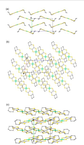
**Figure 6.** Crystal structure of **6** along the (**a**) *a*, (**b**) *b*, and (**c**) *c* axes. Hydrogen atoms are omitted for clarity.
