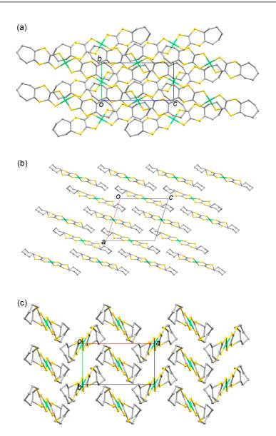
**Figure 8.** Crystal structure of 7 along the (**a**) *a*, (**b**) *b*, and (**c**) *c* axes. Hydrogen atoms are omitted for clarity.
