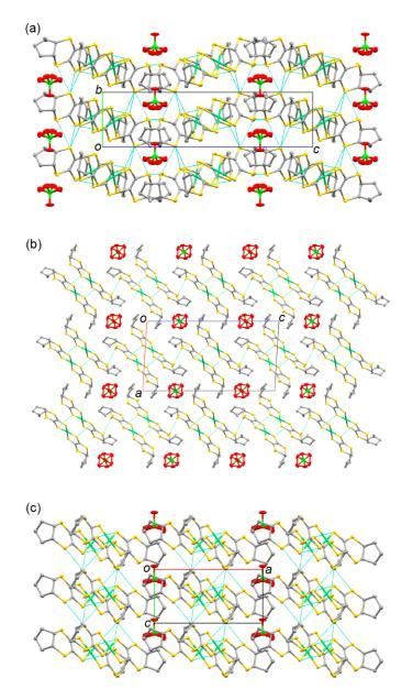
**Figure 14.** Crystal structure of **9** along (**a**) the *a*, (**b**) *b*, and (**c**) *c* axes. Hydrogen atoms are omitted for clarity. The dashed lines indicate sulfur–sulfur distances shorter than the sum of the van der Waals radius (<3.7 Å).
