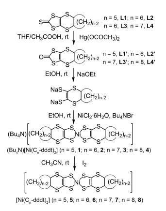
Scheme 3. Synthetic procedure of neutral [Ni(Cn-dddt)<sub>2</sub>] complexes.
