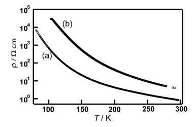
Figure 17. Temperature dependence of electrical resistivities of (a) 9 and (b) 10.
