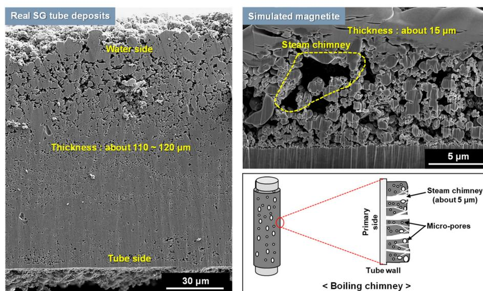
**Figure 8.** Cross-sectional view of the real SG tube deposits and simulated magnetite deposits.
