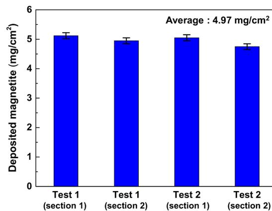
Figure 12. Amount of magnetite deposited onto Alloy 690TT tube.
