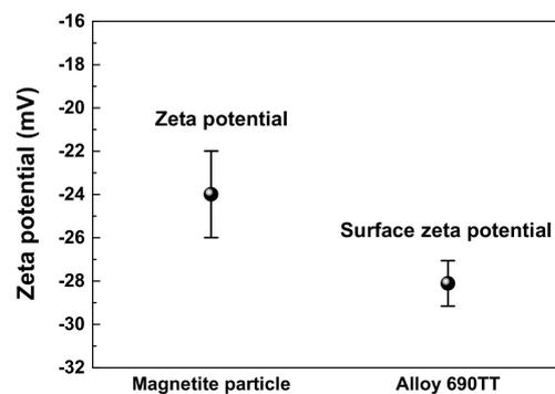
Figure 13. Zeta potentials of magnetite nanoparticle and Alloy 690TT surface.
