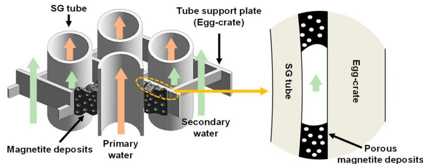
**Figure 1.** Schematic of the secondary flow path between the steam generator (SG) tube and their support plat and tube support plate (TSP) blockage owing to the magnetite deposits.
