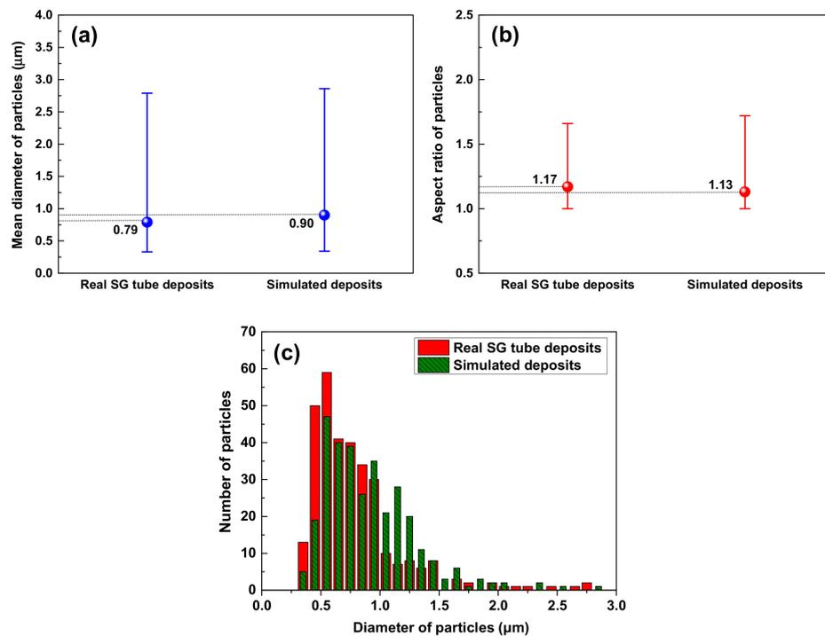
**Figure 7.** Particle size parameters of 320 randomly selected magnetite particles using an image analyzer: (a) mean diameter, (b) aspect ratio, and (c) particle size distribution.
