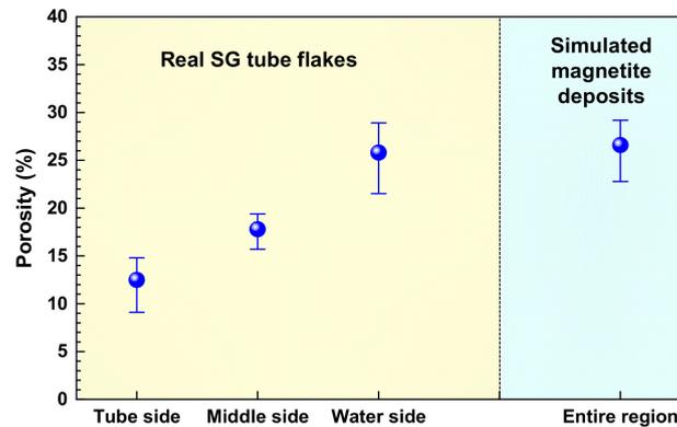
Figure 9. Porosity of the simulated deposit and real SG tube flakes.
