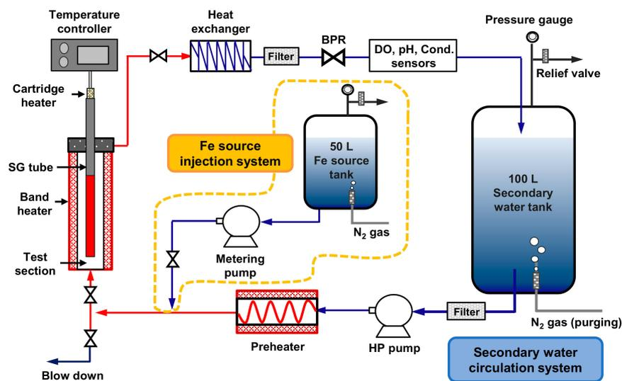
Figure 4. A schematic of the circulation secondary loop system for magnetite deposition test.
