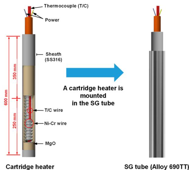
**Figure 2.** Design of cartridge heater and heater-mounted SG tube.
