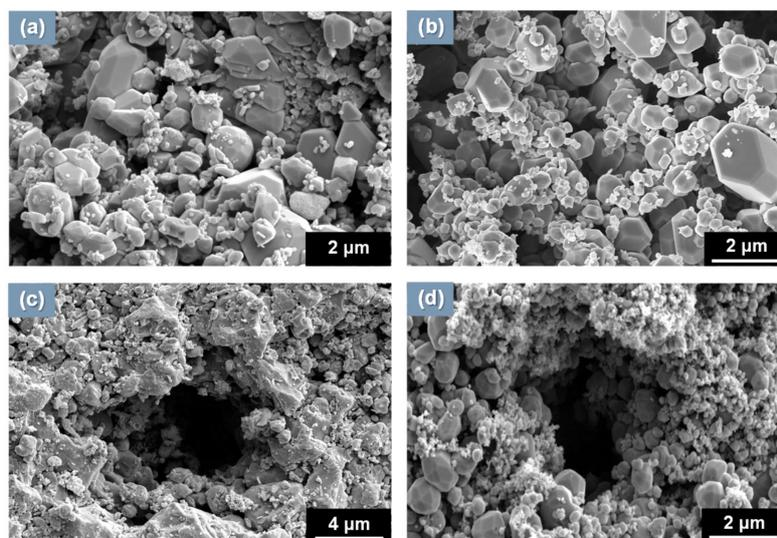
**Figure 6.** Scanning electron microscope (SEM) image of the outer surface of real SG tube deposits and simulated magnetite deposits: (a) particles of real deposits and (b) particles of simulated deposits, (c) pores of real deposits, and (d) pores of simulated deposits.
