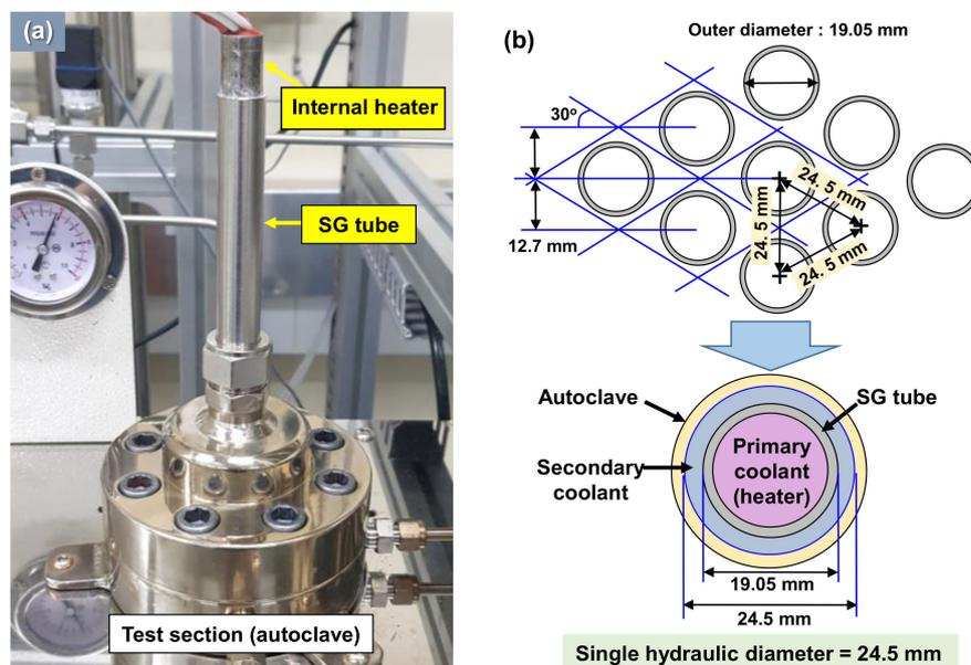
**Figure 3.** (a) Test section and internal heater-mounted SG tube and (b) design of test section as the single hydraulic flow channel.
