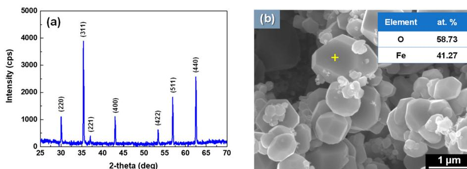
Figure 10. (a) X-ray diffractometer (XRD) pattern of simulated deposit and (b) a representative chemical composition of particle deposited in the test by SEM-energy dispersive X-ray spectrometer (EDS) analysis.
