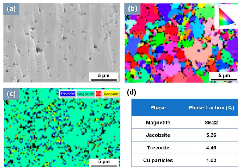
**Figure 11.** Electron back-scatter diffraction (EBSD) data of the real SG tube flake: (a) SEM image, (b) 001 inverse pole figure orientation map, (c) phase distribution map, and (d) relative phase fractions.
