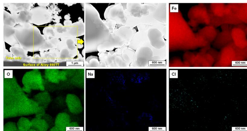
**Figure 14.** Transmission electron microscope (TEM)-EDS mapping analysis of the Na and Cl impurities in the micro-pores formed on the tube side of simulated magnetite deposits.
