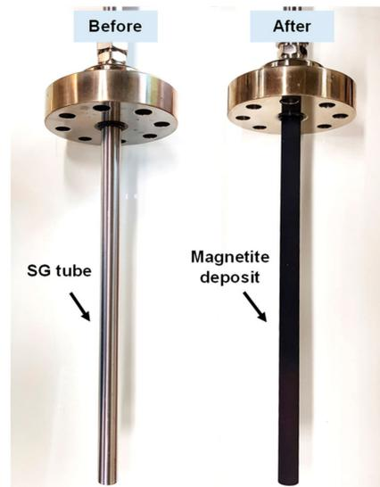
**Figure 5.** Photo of SG tube (Alloy 690TT) before and after the magnetite deposition test.
