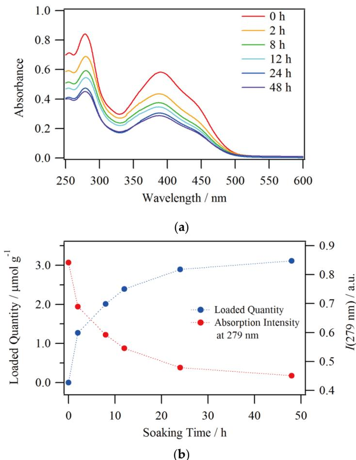
**Figure 5.** Soaking time dependence of (a) UV-Vis absorption spectra and (b) loaded quantity of **1**@Nafion.
