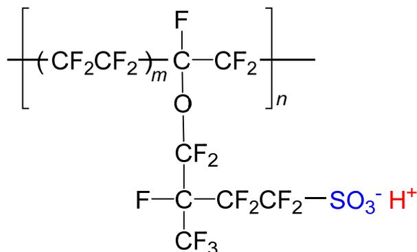
Figure 1. Structural formula of Nafion (acid form).
