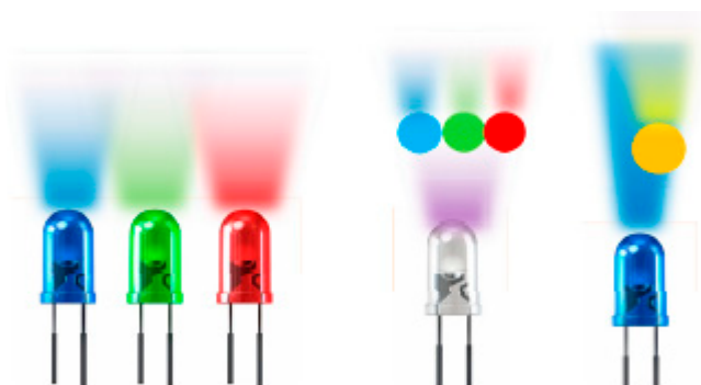
Figure 1. Schematic assembly to obtain white emission in light-emitting diode (LED) technology.
