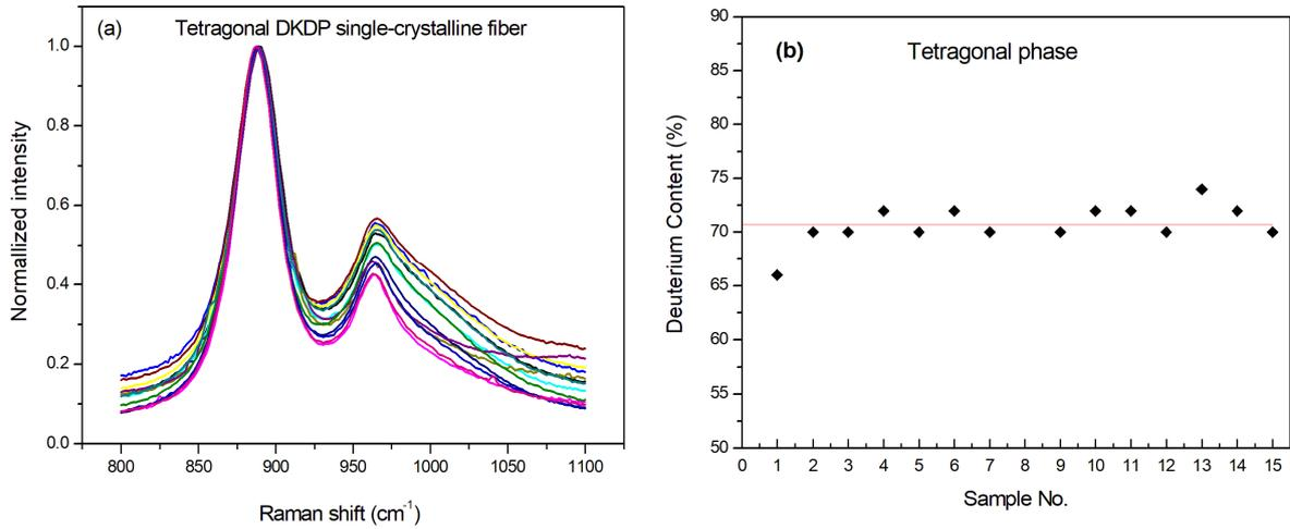
Figure 3. The deuterium content analysis of DKDP tetragonal single-crystalline fibers based on data from seven fiber sample grown in solution containing 85% deuterium. The solid line is the average value of the deuterium-content. The average of the deuterium-content in the tetragonal fiber crystal is about 70.7%.
