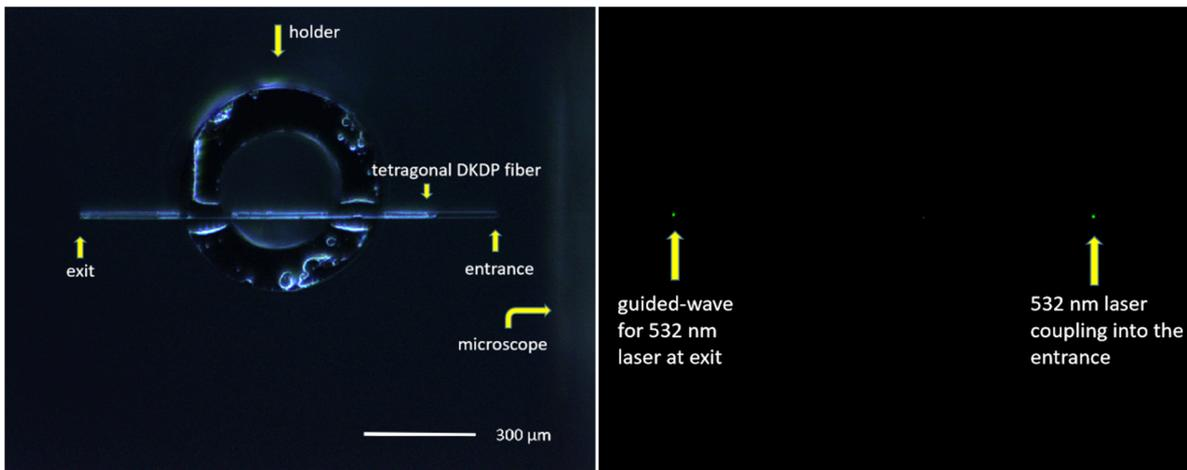
Figure 4. The optical guided-wave for 532 nm laser. The 532 nm laser was coupled to the entrance of a DKDP tetragonal
