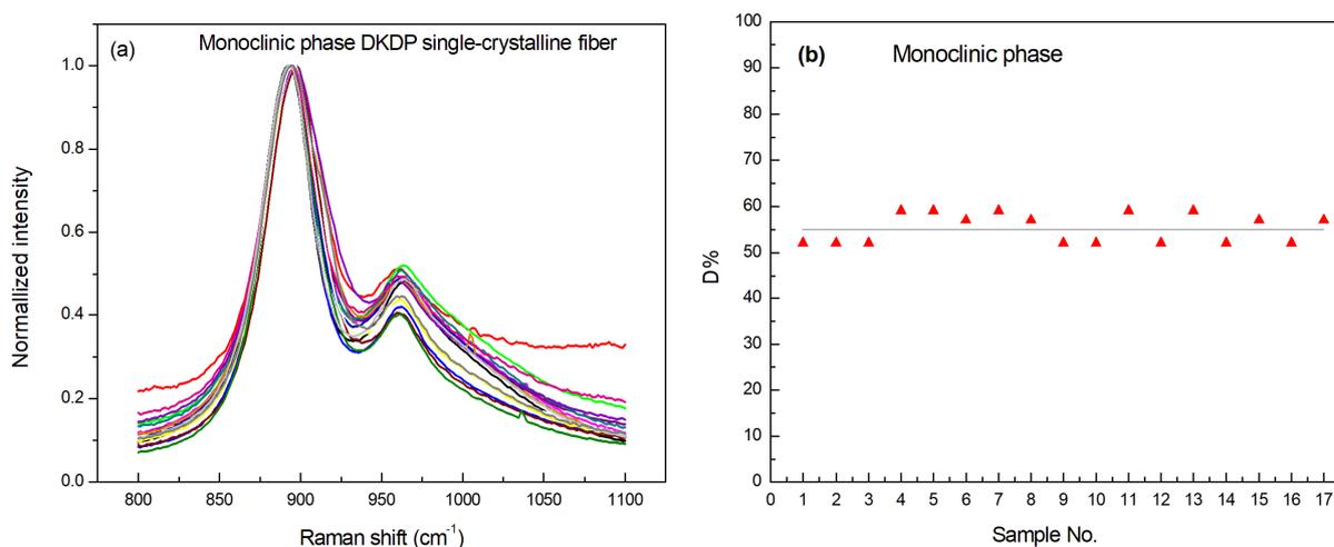
Figure 2. The deuterium content analysis of DKDP monoclinic single-crystalline fibers based on Raman spectra (a) from multiple fiber samples grown in solution containing 75% deuterium (b). The solid line is the average value of the deuterium-content. The average of the deuterium-content in the monoclinic fiber crystal is 55%.
