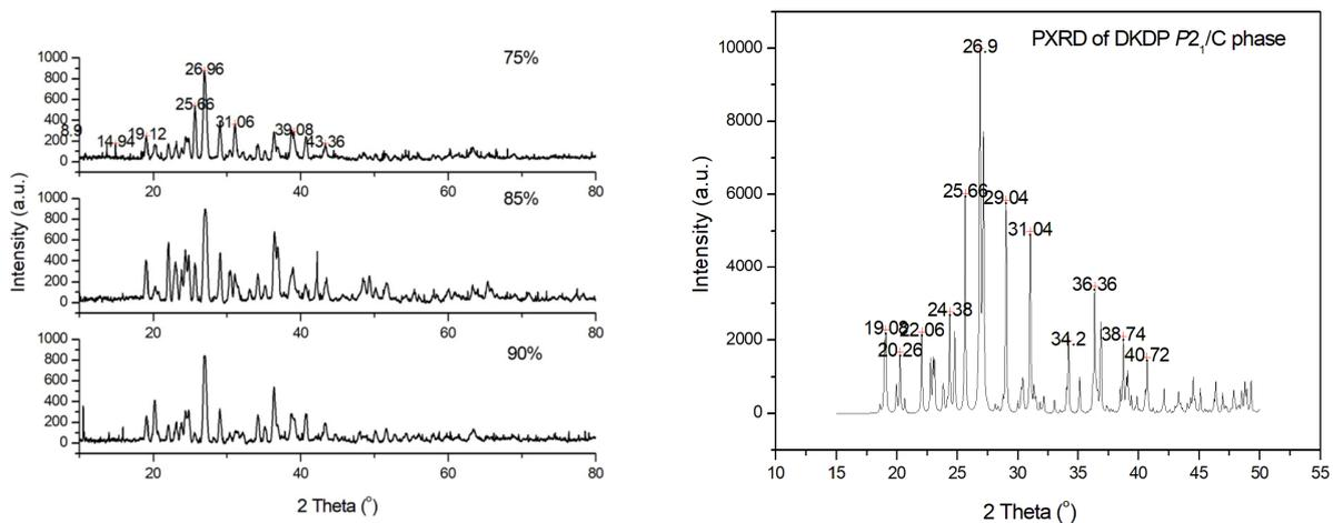
Figure 1. (left) PXR D spectra of the monoclinic DKDP single-crystalline fibers grown in different deuterium-content solution of 75%, 85% and 90%. (right) the theoretical calculated PXR D spectrum based on the structural data file of the monoclinic DKDP single-crystalline fiber.
