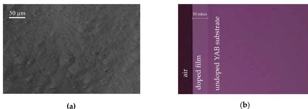
Figure 9. 50\ \mu\text{m} thick as-grown (Er,Yb):YAB layer (a) and polarized optical image of the polished cross-section of the (Er,Yb):YAB layer on the YAB substrate (b).
