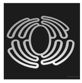
**Figure 2.** Reconstruction of the µ-CT (Micro Computertomography) data of a magnesium scaffold prior to implantation. Bar indicates 5 mm.
