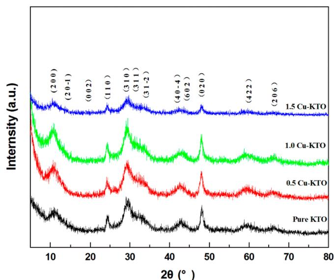
**Figure 1.** XRD spectra of KTO and Cu–KTO nanowires with different Cu doping amounts.
