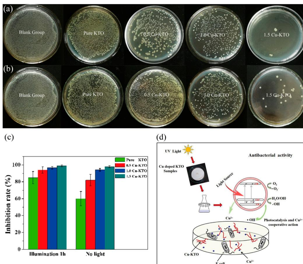
**Figure 7.** The optical images of *E. coli* cultured for 24 h in the presence of different samples irradiated by UV light (a) and without light (b); antibacterial rate (%) against *E. coli* (c); schematic diagram of antibacterial mechanism of Cu–KTO nanowires (d).
