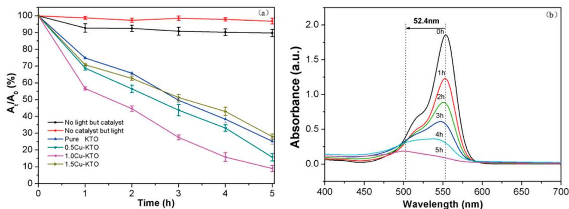
**Figure 6.** Degradation rate of RhB in different conditions with respect to time (a) and UV-Vis absorption spectra of RhB using 1.0 Cu-KTO as the photocatalyst under simulated sunlight irradiation (b).
