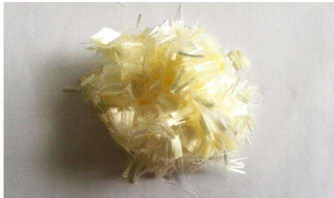
**Figure 2.** PAN fiber for the test.
