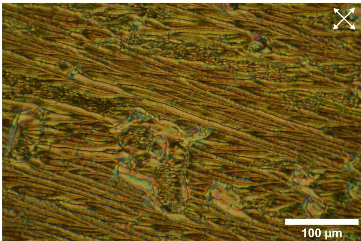
**Figure S4.** POM of the N<sub>TB</sub> phase of a 8CB/CB7CB mixture ( $\phi = 25$  wt%) at -20°C. Crossed polarizers.
