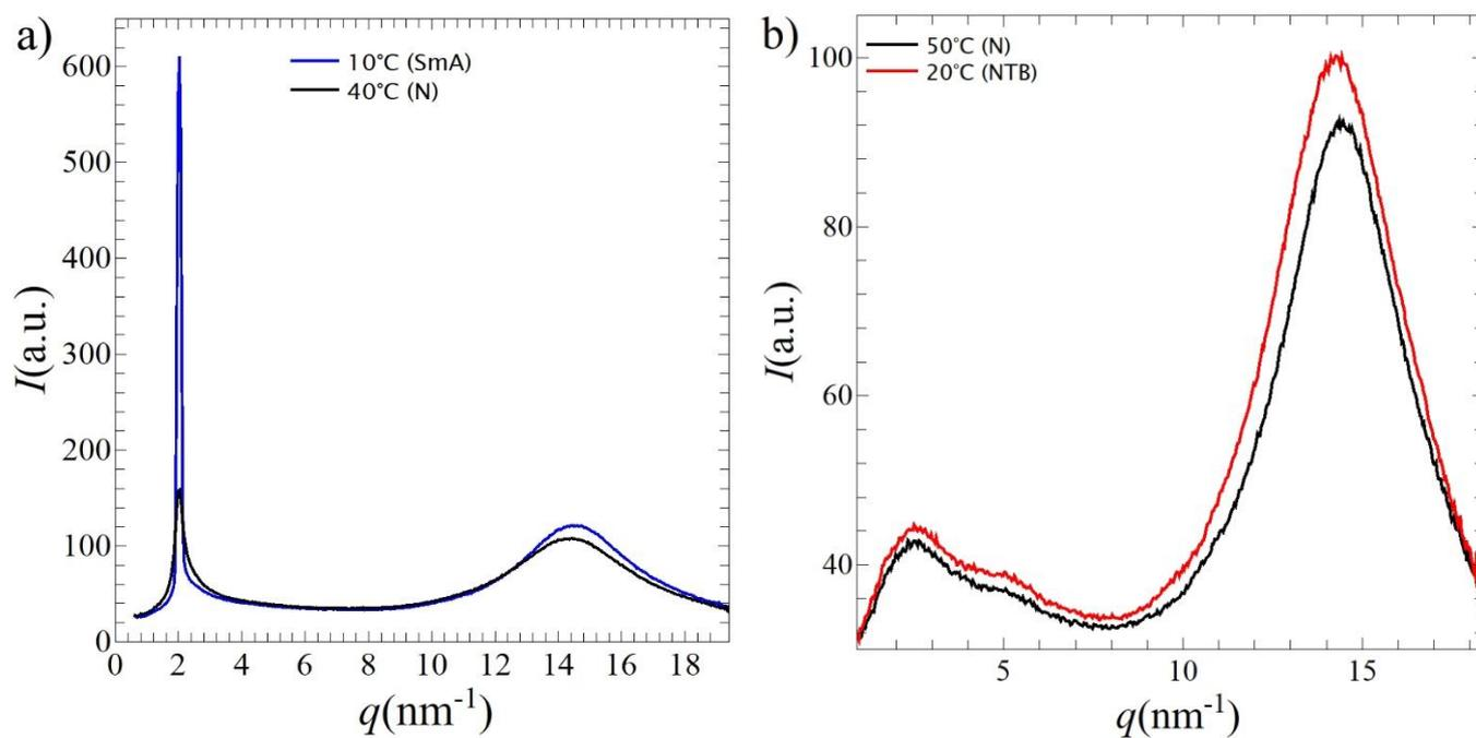
**Figure S3.** X-rays diffracted intensities of 8CB/CB7CB mixtures as a function of wave vector  $q$ . **(a)** Mixture at a concentration  $\phi = 10.3$  wt% of CB7CB in SmA phase at 10°C and in N phase at 40°C. **(b)** Mixture at a concentration  $\phi = 54.9$  wt% of CB7CB in N<sub>TB</sub> phase at 20°C and N phase at 50°C.
