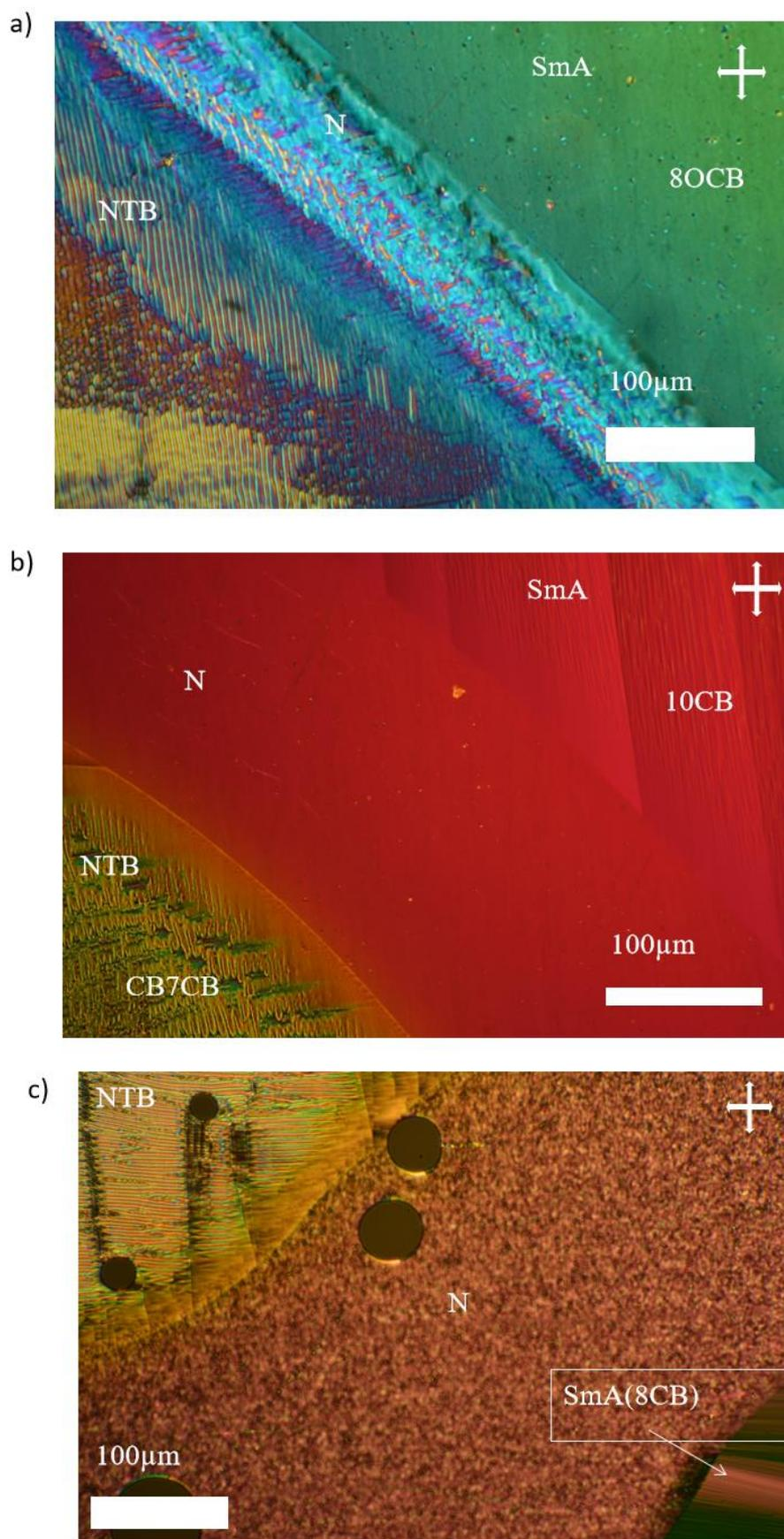
**Figure S5** Contact experiments at room temperature of various smectogens -(a) 8OCB, (b) 10CB, (c) 8CB- with CB7CB. In the vicinity of the contact we never observed a  $N_{TB}/SmA$  front interface but the sequence  $SmA-N-N_{TB}$  phases (POM).
