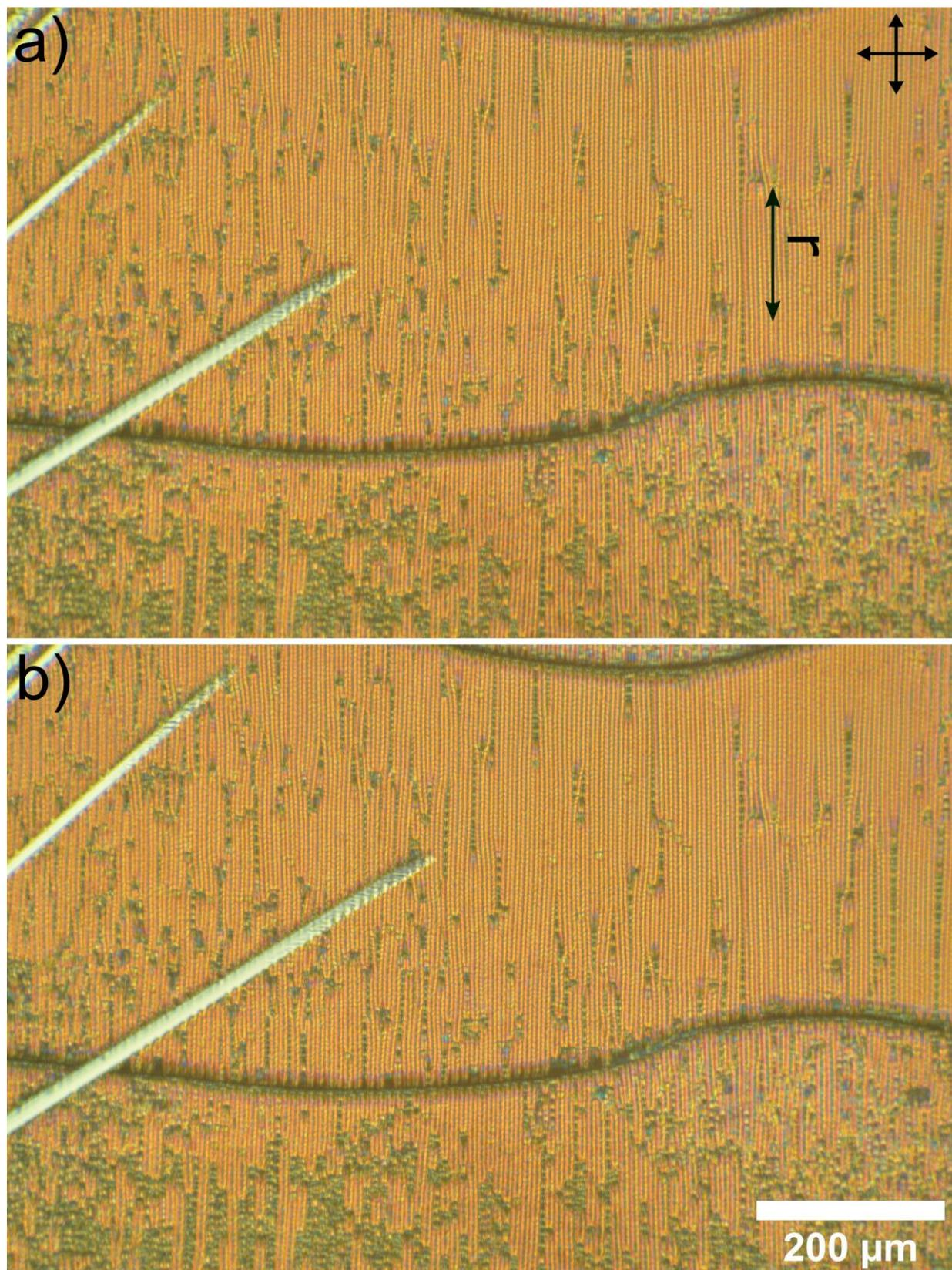
**Figure S2.** (a) Growth of needle crystals in the  $N_{TB}$  phase of CB7CB at 95°C in a planar cell (EHC, thickness 10μm). The crystallization was induced by a CB7CB crystal seed in contact with the periphery of the cell (at a distance about 10mm). (b) Image of the same region taken 1 min later. The crystal growth velocity is thus about 100μm.min<sup>-1</sup> and the cell totally crystallizes in several hours. Crossed polarizers, r indicates the rubbing direction.
