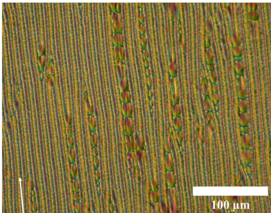
**Figure S9.** POM texture at room temperature of the 8CB/CB7CB binary system at a concentration  $\phi = 50$  wt%. The N<sub>TB</sub> phase shows the typical stripes and ropes textures. Planar anchoring: the arrow indicates the rubbing direction of the PVA layers.
