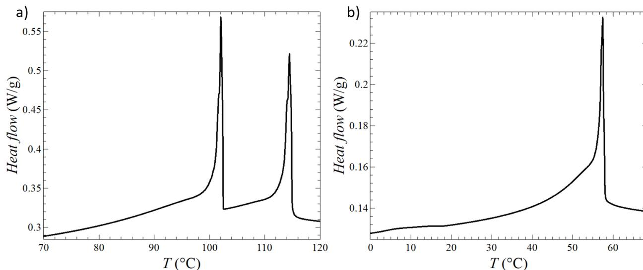
**Figure S8.** (a) Heat flow curve of pure CB7CB is characterized by two distinct peaks of similar magnitude corresponding respectively to the Iso/N and N/N<sub>TB</sub> phase transitions. (b) A mixture at concentration  $\phi=43$  wt% still displays a strong Iso/N phase transition peak but the N/N<sub>TB</sub> one is barely visible, in the shape of a broad weak hump.
