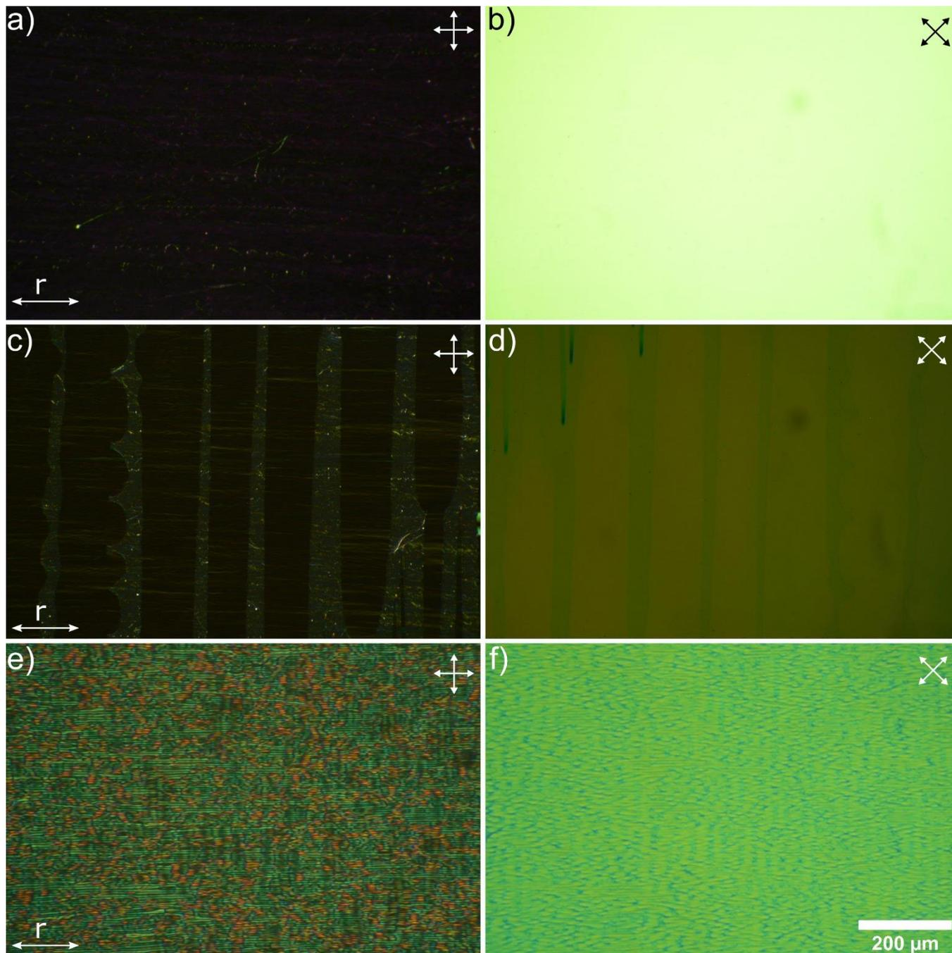
**Figure S1.** Polarizing optical micrographs of CB7CB observed at different temperatures in a planar cell (EHC, 10 $\mu$ m). (a) and (b) Nematic phase at 105°C. (c) and (d) Multiples domains of N<sub>TB</sub> phase appearing in the N phase during the N/ N<sub>TB</sub> transition at 104°C. The difference between the two phases is quite visible. (e) and (f) N<sub>TB</sub> phase observed at 102°C. Crossed polarizers, r indicates the rubbing direction.
