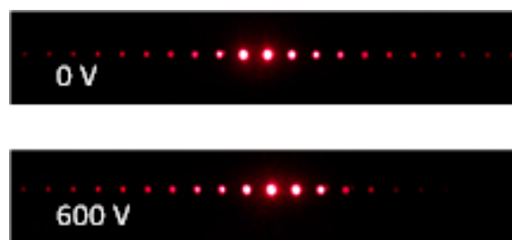
Figure 25. Laser beam ( \lambda = 633 nm) steering patterns without and with applied voltages. Reproduced with permission [91]. Copyright 2017, Photonics Society of Poland.
