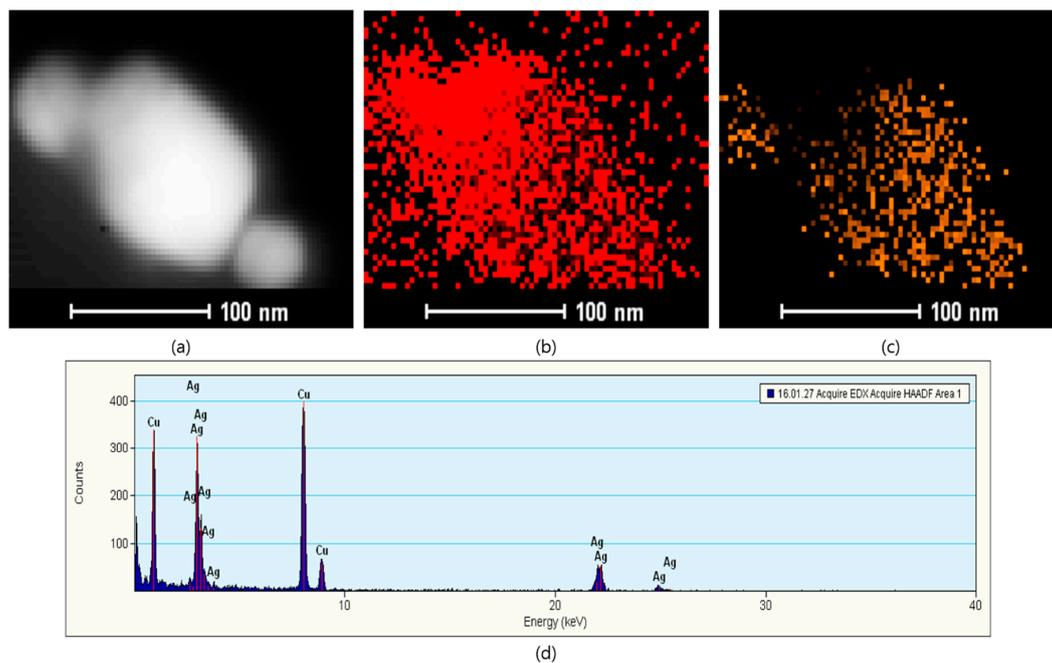
**Figure 4.** STEM-HAADF, elemental mapping, and EDX spectrum of copper-silver bimetallic nanostructures: (a) STEM-HAADF image; (b) copper; (c) silver; and, (d) EDX spectrum.
