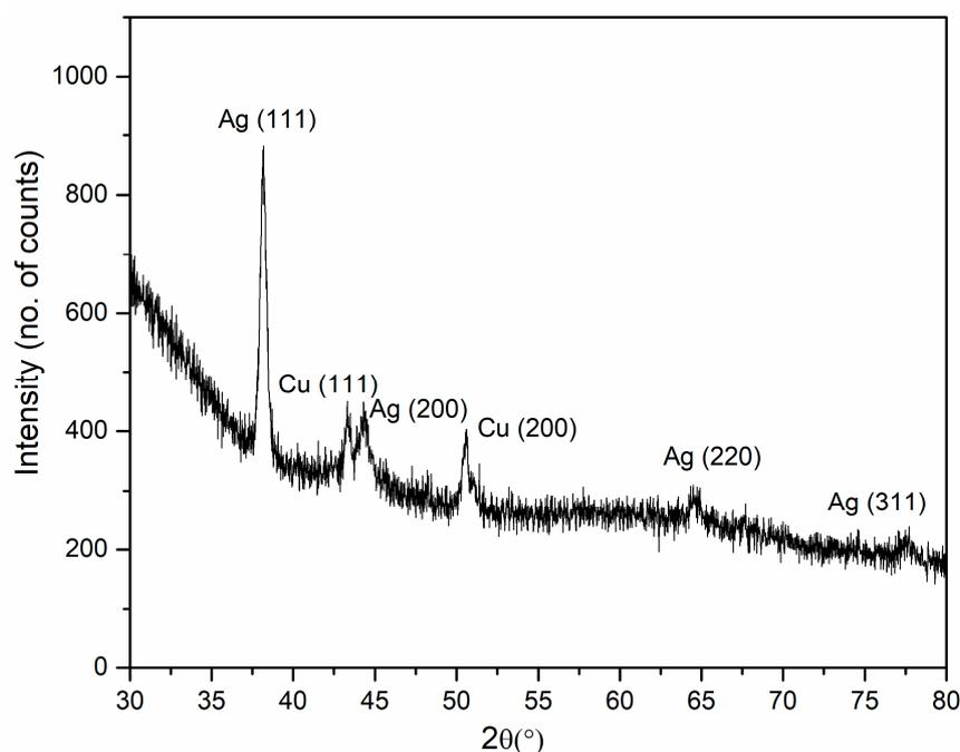
Figure 2. XRD spectrum of copper-silver bimetallic nanostructures.
