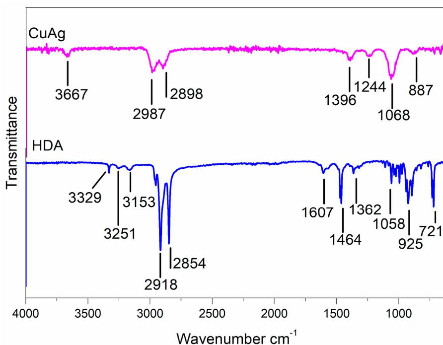
Figure 5. FTIR spectra of copper-silver bimetallic nanostructures and hexadecylamine.
