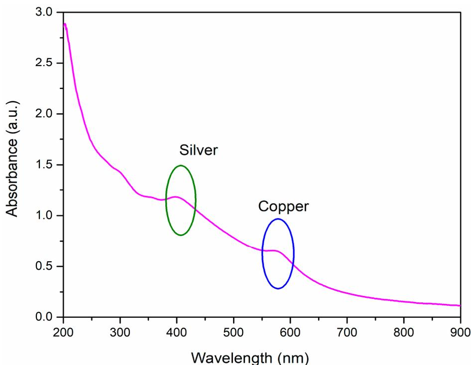
**Figure 1.** UV-Vis spectra of copper-silver bimetallic nanostructures.
