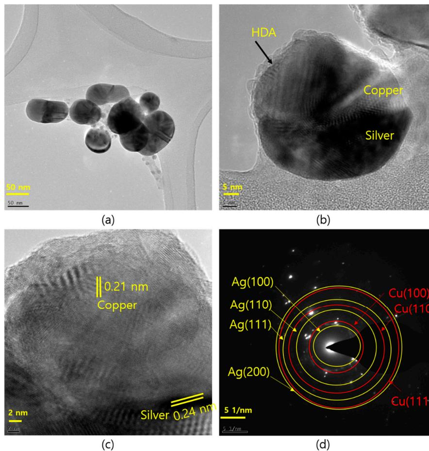
**Figure 3.** Different magnification HR-TEM images of copper-silver bimetallic nanostructures: (a) 100 nm; (b) representing the silver and copper nanoparticles with hexadecylamine (had) layer; (c) lattice fringes of Cu-Ag nanoparticle; and, (d) SAED pattern of Cu-Ag nanoparticles.
