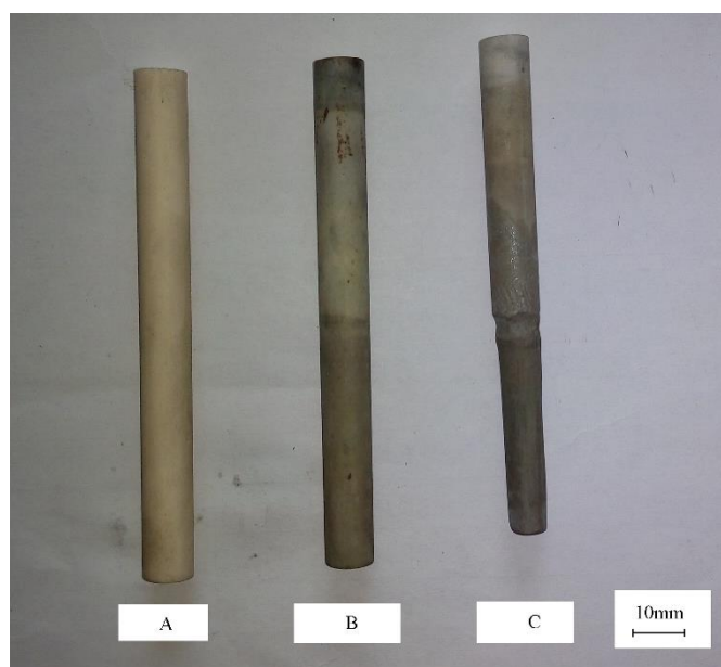
Figure 2. \text{Al}_2\text{O}_3 rods before and after dissolution experiments: (A)—Original rod; (B)—Base slag, w(\text{CaO}):w(\text{Al}_2\text{O}_3) = 1:2 ; (C)— w(\text{CaF}_2) = 20\% , w(\text{CaO}):w(\text{Al}_2\text{O}_3) = 1:2 .
