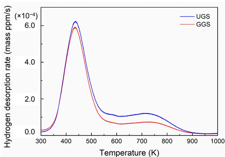
**Figure 4.** TDA spectra of the investigated steels after hydrogen charging at a current density of  $30 \text{ A}\cdot\text{m}^{-2}$  for 6 h at 360 K.
