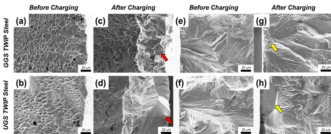
**Figure 3.** Fracture surface of the investigated materials in the (a–d) monotonic and (e–h) cyclic deformation modes. The images were obtained (a,b,e,f) before and (c,d,g,h) after hydrogen charging at a current density of  $30 \text{ A}\cdot\text{m}^{-2}$  for 6 h at 360 K.
