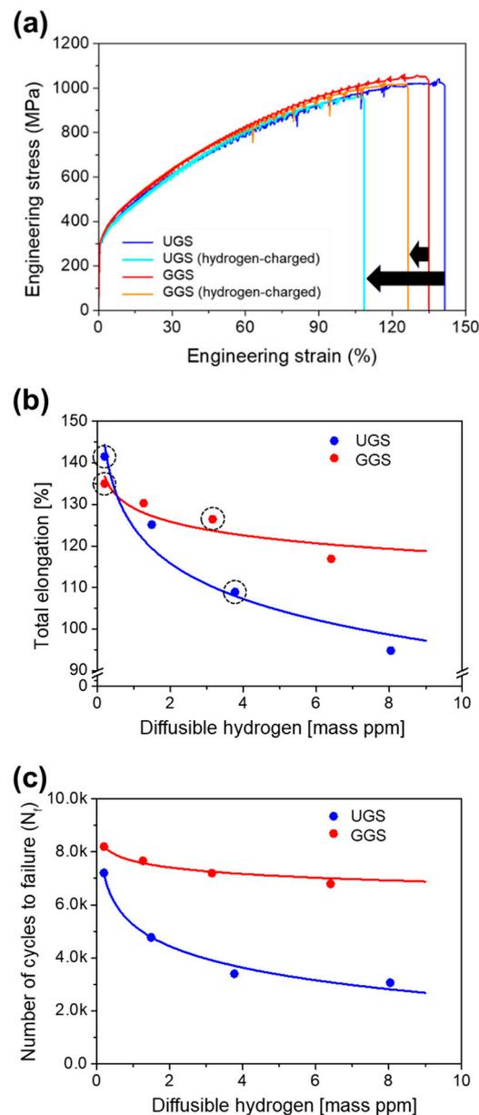
**Figure 2.** Variation in mechanical behaviors after hydrogen charging in the (a,b) monotonic and (c) cyclic deformation modes. Engineering stress–strain curves in Figure 2a correspond to the data points marked by the dotted circles in Figure 2b. In Figure 2a, hydrogen was charged at a current density of  $30 \text{ A}\cdot\text{m}^{-2}$  for 6 h at 360 K.
