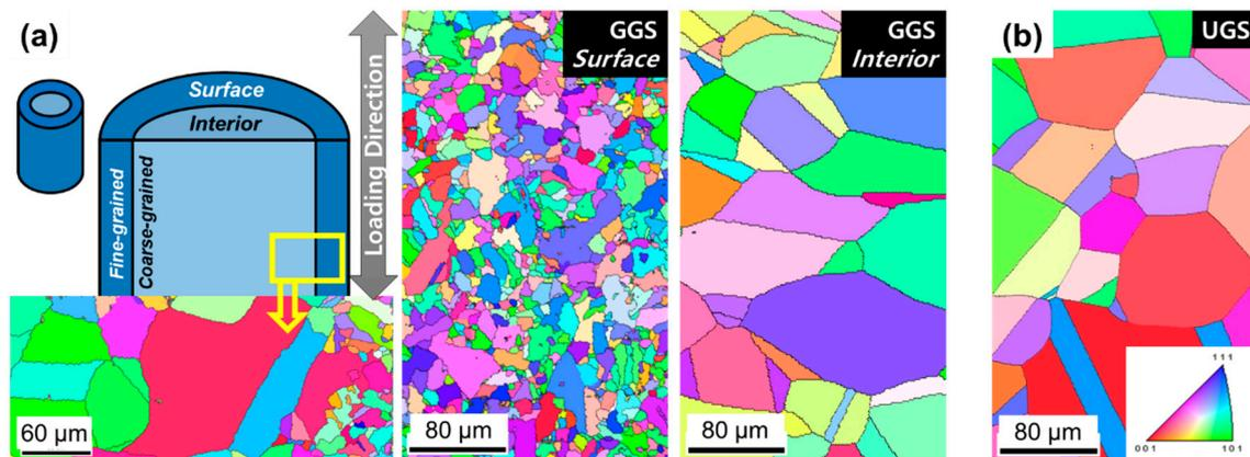
**Figure 1.** Electron backscatter diffraction (EBSD) inverse pole figure map of (a) GGS and (b) UGS TWIP steels. The images are perpendicular to the normal direction.
