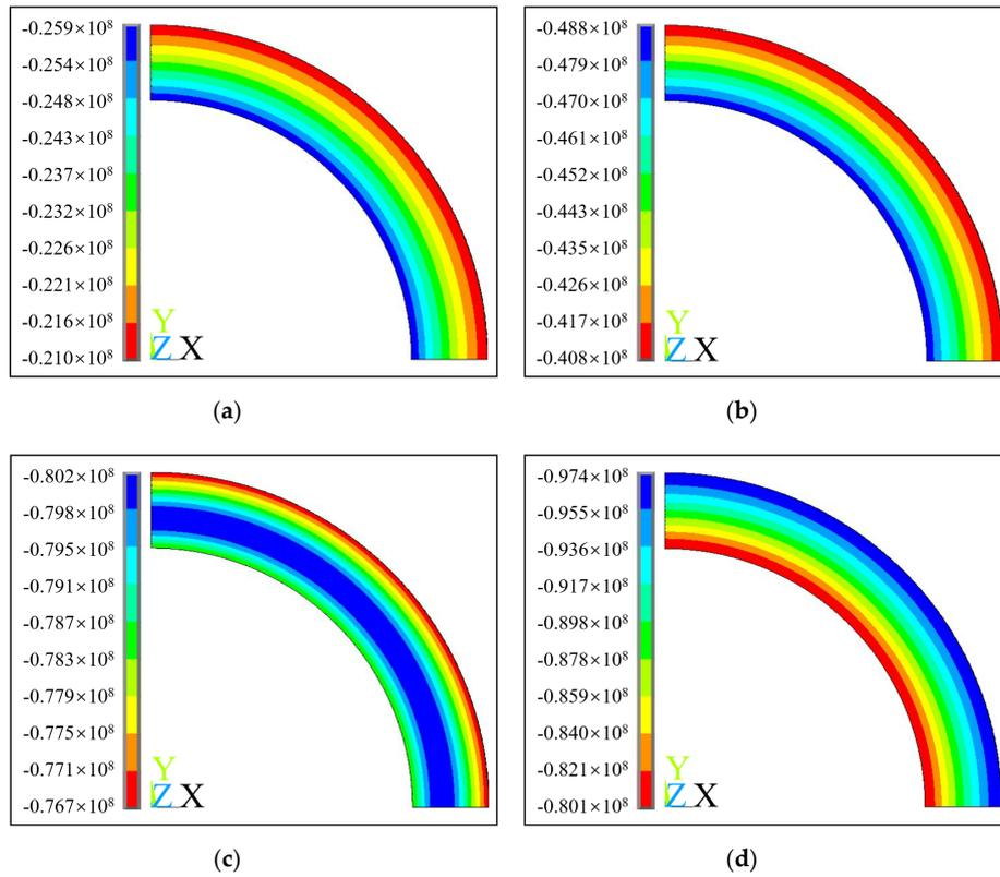
**Figure 4.** Hoop stress cloud diagrams of D-5 model shaft lining concrete under a surface load: (a) 5 MPa; (b) 10 MPa; (c) 18 MPa; (d) 23.3 MPa.
