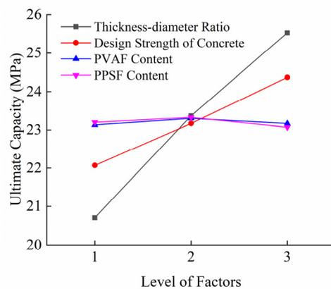
**Figure 14.** Relation curve of each factor and ultimate capacity of the shaft lining structure.
