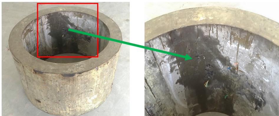
**Figure 12.** The failure mode of the HFRC shaft lining model.
