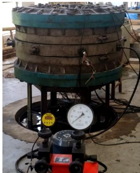
**Figure 11.** Shaft lining structure high-pressure loading device.
