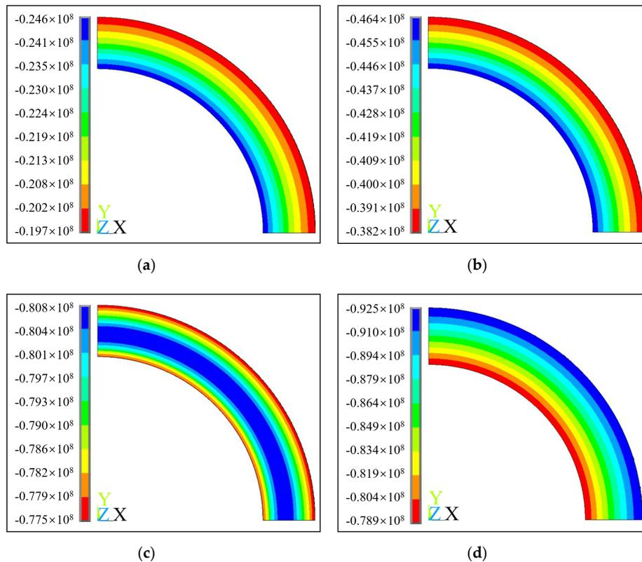
**Figure 5.** Hoop stress cloud diagrams of D-8 model shaft lining concrete under a surface load: (a) 5 MPa; (b) 10 MPa; (c) 19 MPa; (d) 25.3 MPa.
