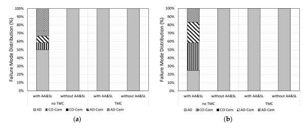
**Figure 6.** Failure modes of the specimens for (**a**) Shofu HC Hard (SH) and (**b**) Cerasmart 300 (CE) after the shear bond strength tests. AA&SL: alumina air-abraded and silanized specimen. TMC: 20,000-thermocycled specimen. No-TMC: 0-thermocycled specimen. AD: adhesive failure, CO-Com: cohesive failure in composite, CO-Cem: cohesive failure in cement, AD-Com: mixed failure adhesive + cohesive in composite, AD-Cem: mixed failure adhesive + cohesive in cement.
