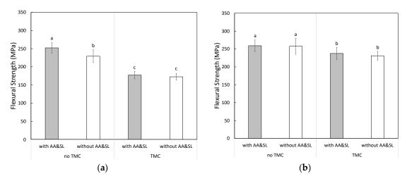
**Figure 4.** Mean flexural strength values of the bonded-double-bar specimens for (**a**) Shofu HC Hard (SH) and (**b**) Cerasmart 300 (CE), as illustrated in Figure 1b. The vertical error-bars indicate standard deviations. The different letters indicate a significant difference between the groups (p < 0.05, Tukey test, n = 12). AA&SL: alumina air-abraded and silanized specimen. TMC: 20,000-thermocycled specimen. No-TMC: 0-thermocycled specimen.
