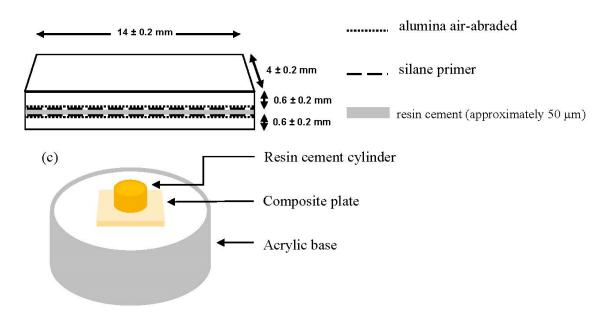
**Figure 1.** Specimen designs and dimensions for three-point bending tests with (**a**) single-bar, (**b**) bonded-double-bar, and (**c**) for shear bond strength (SBS) test with cylindrical specimen.
