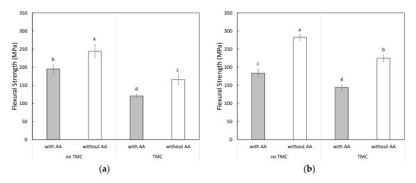
**Figure 3.** Mean flexural strength values of the single-bar specimens for (**a**) Shofu HC Hard (SH) and (**b**) Cerasmart 300 (CE), as illustrated in Figure 1a. The vertical error-bars indicate standard deviations. The different letters indicate a significant difference between the groups (p < 0.05, Tukey test, n = 12). AA: alumina air-abraded specimen. TMC: 20,000-thermocycled specimen. No-TMC: 0-thermocycled specimen.
