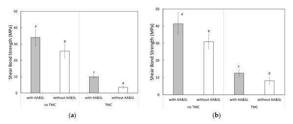
**Figure 5.** Shear bond strength of the specimens for (**a**) Shofu HC Hard (SH) and (**b**) Cerasmart 300 (CE), as illustrated in Figure 1c. The vertical error-bars indicate standard deviations. The different letters indicate a significant difference between the groups (p < 0.05, Tukey test, n = 12). AA&SL: alumina air-abraded and silanized specimen. TMC: 20,000-thermocycled specimen. No-TMC: 0-thermocycled specimen.
