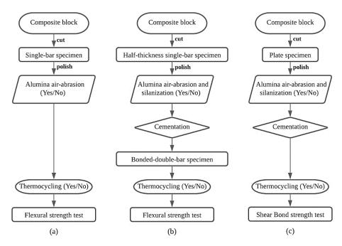
**Figure 2.** Protocol diagrams of the sample preparation and testing procedures for: (**a**) flexural strength testing for single-bar specimen; (**b**) flexural strength testing for bonded-double-bar specimen; (**c**) shear bond strength testing.
