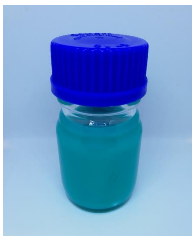
Figure A1. A mixture of 1.6 g \text{Cu}(\text{OAc})_2 \cdot \text{H}_2\text{O} and 1.5 g OH- m BDC in 100 mL DMSO after 2 h, showing a precipitation occurred in [\text{Cu}_{24}(\text{OH-}m\text{BDC})_{24}]_n stock solution.
