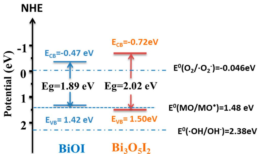
Figure S2. The energy band structure of Bi<sub>3</sub>O<sub>5</sub>I<sub>2</sub> and BiOI.
