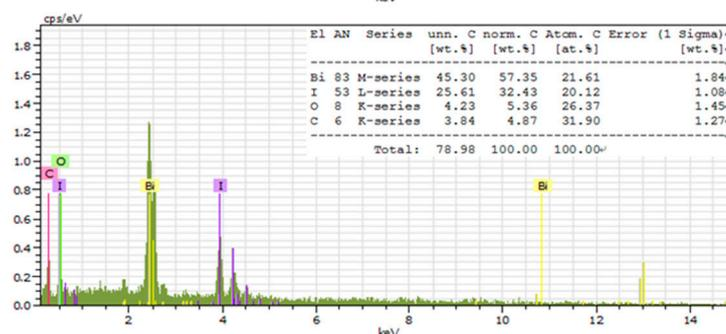
Figure S1. SEM images and EDS analysis of as prepared samples in different locations: (a), (b) I-poor bismuth oxyiodide, (c), (d)BiOI.
