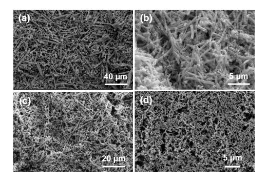
**Figure S2**. Scanning electron microscope images of copper-platinum macrotube structures from DMAB reduced salts with Pt<sup>2-</sup>:Pt<sup>2+</sup>:Cu<sup>2+</sup> ratios of (**a**) 1:0:1, (**b**) 3:1:2, (**c**) 2:1:1, and (**d**) 1:1:0.
