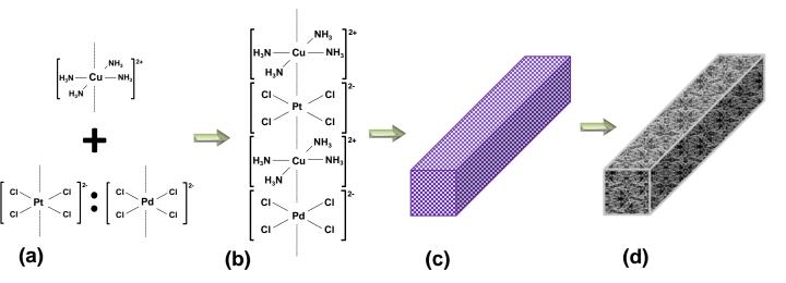
**Figure S1. Macrobeam synthesis scheme**. (a) Addition of  $[PtCl_4]^{2-}$  and  $[PdCl_4]^{2-}$  with  $[Cu(NH_3)_4]^{2+}$ . (b) Linear stacking of platinum and copper square planar complex ions. (c) Formation of Magnus's salt crystal derivatives. (d) Reduction of platinum/palladium-copper salt needle template to square cross-section macrobeam.
