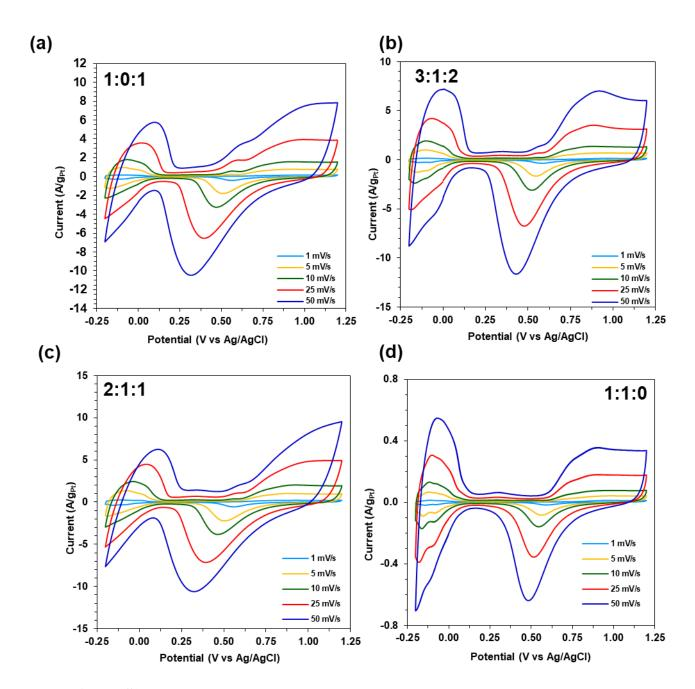
**Figure S8**. Cyclic voltammetry (CV) curves of platinum-copper macrobeams from DMAB reduced salts with  $Pt^{2-}:Pt^{2+}:Cu^{2+}$  ratios of (a) 1:0:1, (b) 3:1:2, (c) 2:1:1, and (d) 1:1:0 in 0.5 M  $H_2SO_4$  at scan rates of 1, 5, 10, 25, and 50 mV/s.
