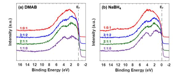
**Figure S6.** X-ray photoelectron spectra (XPS) valence-band spectra (VBS) of the Pt–Cu macrobeams from (**a**) DMAB, and (**b**) NaBH<sub>4</sub> reduced salts with Pt<sup>2-</sup>:Pt<sup>2+</sup>:Cu<sup>2+</sup> ratios of 1:0:1, 3:1:2, 2:1:1, and 1:1:0.
