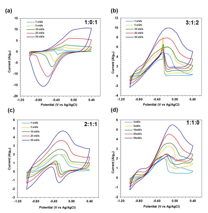
**Figure S11**. Cyclic voltammetry (CV) curves of platinum-copper macrobeams from NaBH<sub>4</sub> reduced salts with Pt<sup>2-</sup>:Pt<sup>2+</sup>:Cu<sup>2+</sup> ratios of (**a**) 1:0:1, (**b**) 3:1:2, (**c**) 2:1:1, and (**d**) 1:1:0 in 1 M KOH and 1 M ethanol at scan rates of 1, 5, 10, 25, and 50 mV/s.
