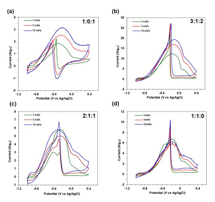
**Figure S9**. Cyclic voltammetry (CV) curves of platinum-copper macrobeams from DMAB reduced salts with Pt<sup>2-</sup>:Pt<sup>2+</sup>:Cu<sup>2+</sup> ratios of (**a**) 1:0:1, (**b**) 3:1:2, (**c**) 2:1:1, and (**d**) 1:1:0 in 1 M KOH and 1 M ethanol at scan rates of 1, 5, and 10 mV/s.
