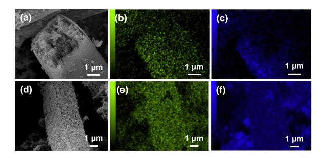
**Figure S5**. Energy dispersive X-ray spectroscopy mapping of platinum-copper macrobeams from salts with a Pt<sup>2-</sup>:Pt<sup>2+</sup>:Cu<sup>2+</sup> ratio of 1:0:1 reduced with (**a-c**) DMAB and (**d-f**) NaBH<sub>4</sub>. (**b,e**) Cu-K line (green), and (**c,f**) Pt-M line (blue) mapped.
