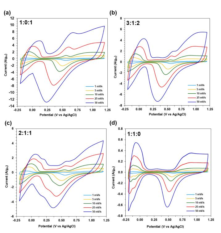
**Figure S10**. Cyclic voltammetry (CV) curves of platinum-copper macrobeams from NaBH<sub>4</sub> reduced salts with Pt<sup>2-</sup>:Pt<sup>2+</sup>:Cu<sup>2+</sup> ratios of (**a**) 1:0:1, (**b**) 3:1:2, (**c**) 2:1:1, and (**d**) 1:1:0 in 0.5 M H<sub>2</sub>SO<sub>4</sub> at scan rates of 1, 5, 10, 25, and 50 mV/s.
