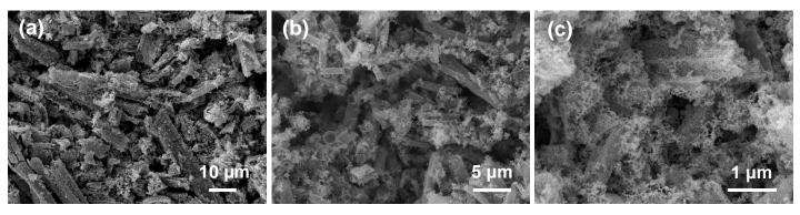
**Figure S3**. Scanning electron microscope images of copper-platinum macrobeam structures from NaBH<sub>4</sub> reduced salts with Pt<sup>2-</sup>:Pt<sup>2+</sup>:Cu<sup>2+</sup> ratios of (**a**) 1:0:1, (**b**) 3:1:2, and (**c**) 2:1:1.
