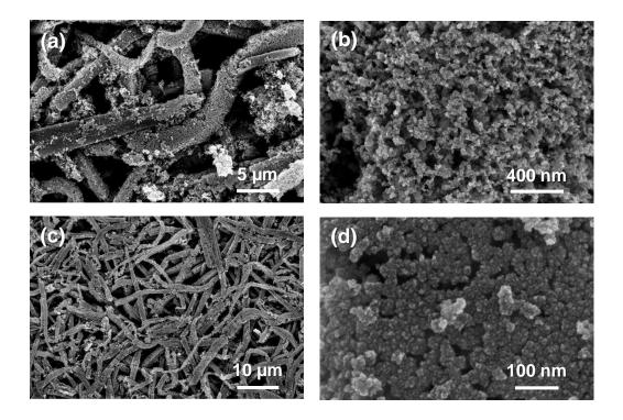
**Figure S4**. Scanning electron microscope images of platinum-copper macrobeams from DMAB reduced salts with  $Pt^{2-}$ : $Pd^{2+}$ : $Cu^{2+}$  ratios of  $(\mathbf{a},\mathbf{b})$  2:1:1, and  $(\mathbf{c},\mathbf{d})$  3:1:2.
