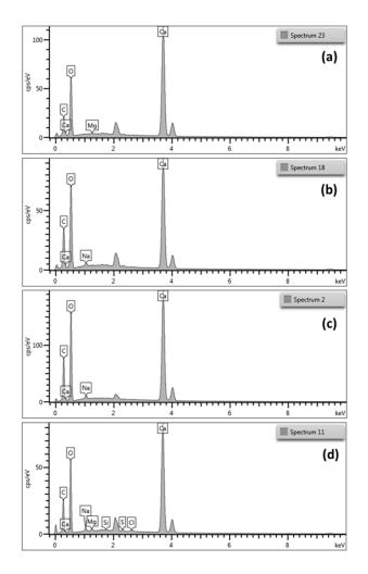
Figure S2. SEM-EDS data of catalysts before calcination. (a) commercial CaO; (b) S-shell; (c) C-shell; (d) O-shell.
