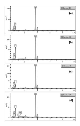
**Figure S3.** SEM-EDS data of catalysts after calcination at 950 °C. (**a**) commercial CaO; (**b**) S-shell-950; (**c**) C-shell-950; (**d**) O-shell-950.
