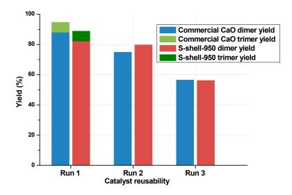
**Figure S1.** Catalyst reusability of commercial CaO and S-shell-950 catalysts. Reaction conditions: 4.0 g cyclopentanone; 1.0 g catalyst; 180 °C; 2h. Catalysts were regenerated by calcination at 950 °C for 4 h.
