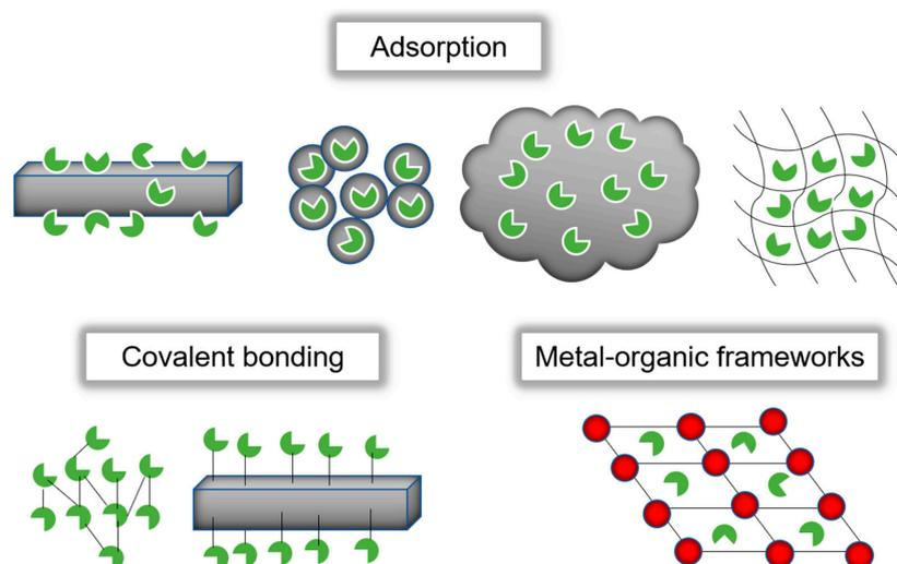
Figure 1. Schematic of various carriers for immobilization of enzymes.
