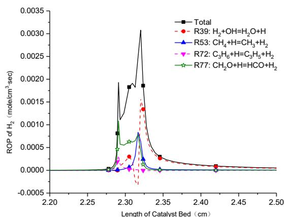
Figure 8. ROP analysis of  $H_2$  concentration in the preferred reaction conditions.
