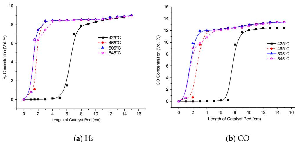
**Figure 3.** Reaction temperature effect on H<sub>2</sub> and CO concentration.
