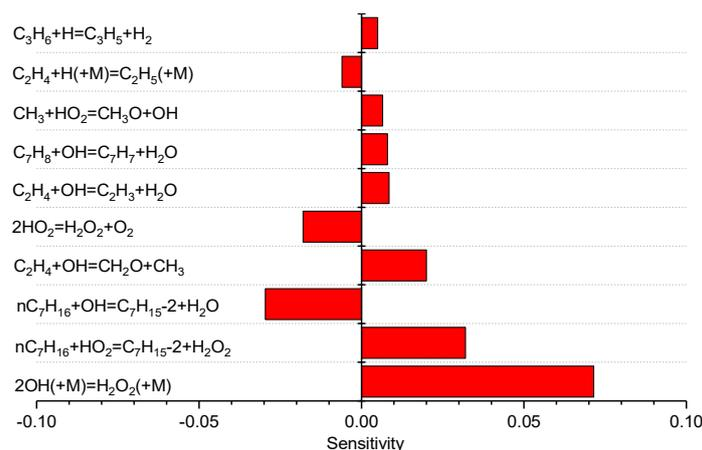
Figure 7. Sensitivity analysis of  $H_2$  concentration in the preferred reaction conditions.
