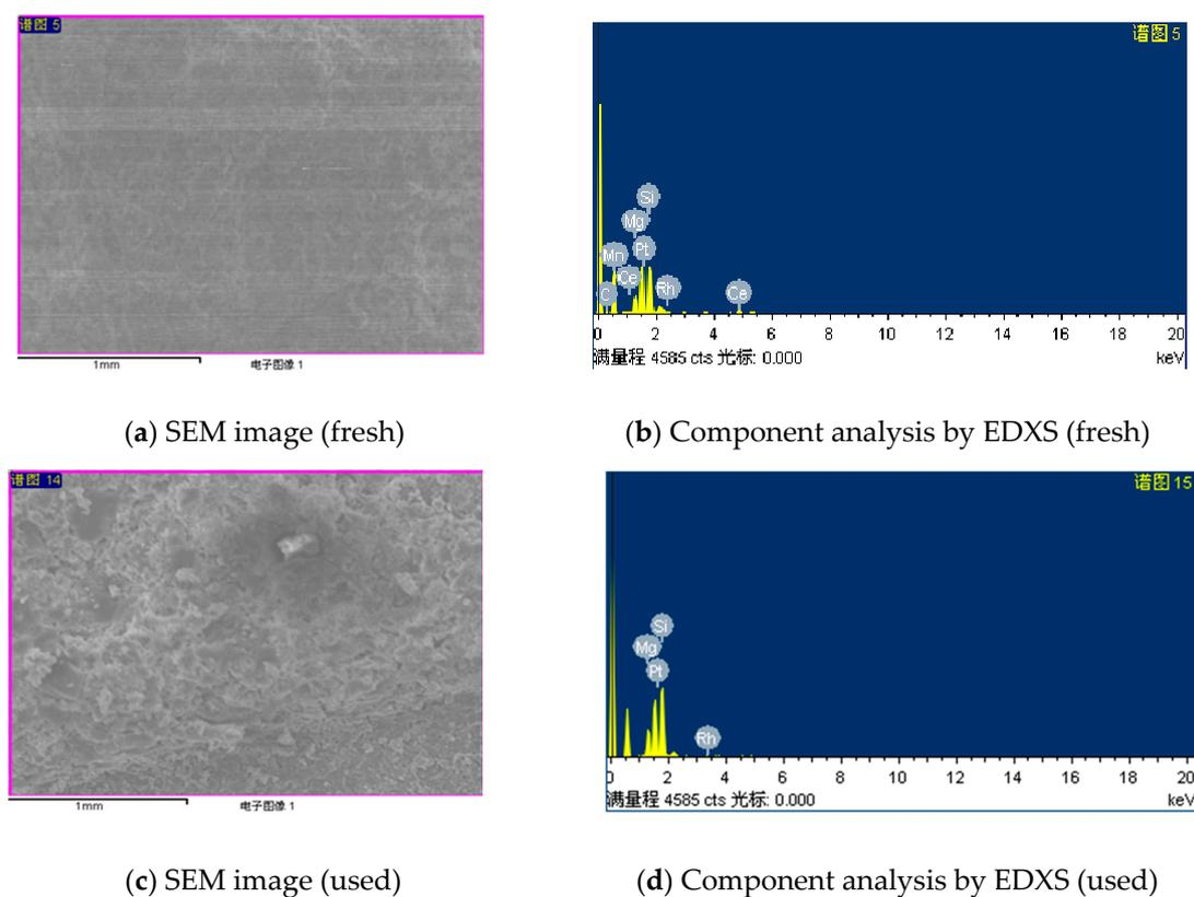
**Figure 9.** SEM/EDXS analysis of an advanced TWC sample (fresh and used catalysts).
