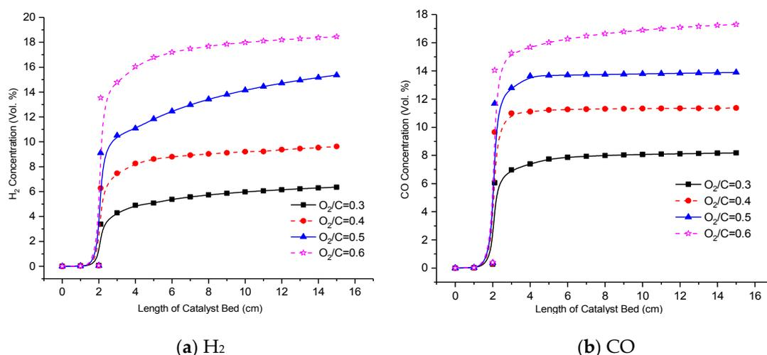
Figure 6. O<sub>2</sub>/C ratio effect on H<sub>2</sub> and CO concentration.
