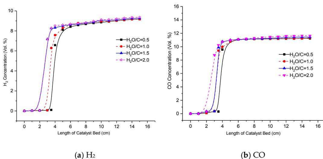
Figure 5. H<sub>2</sub>O/C ratio effect on H<sub>2</sub> and CO concentration.
