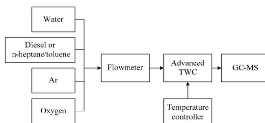
Figure 2. Schematic of reforming experimental setup.
