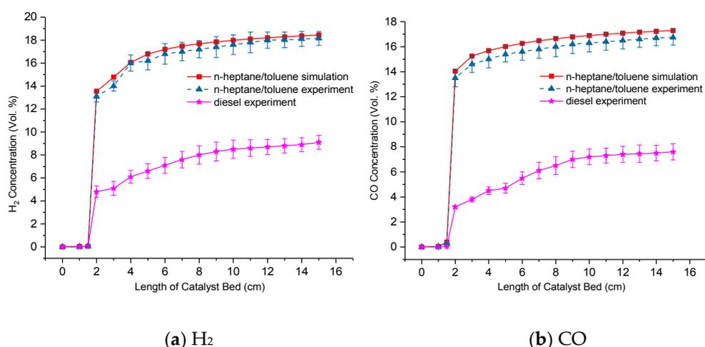
**Figure 12.** H<sub>2</sub> and CO concentration comparison and Error bars analysis.
