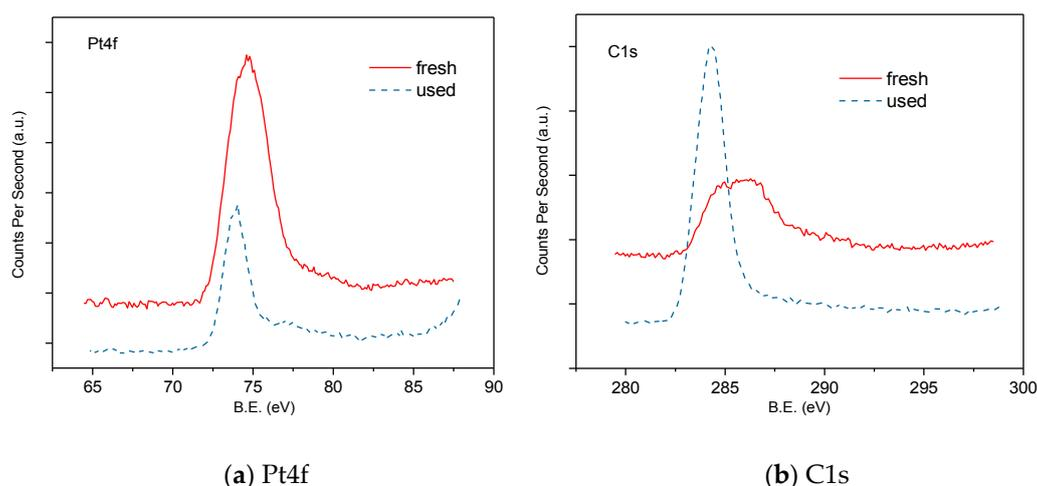
**Figure 11.** XPS patterns of Pt4f and C1s photoemission spectra of the Pt/Rh TWC catalysts.
