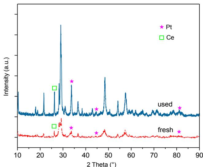
**Figure 10.** XRD patterns of Pt/Rh TWC catalysts for  $2\theta$  between  $10^\circ$  and  $90^\circ$  in the fresh state and after the used state.
