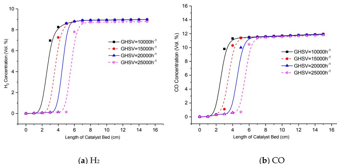
Figure 4. GHSV effect on H<sub>2</sub> and CO concentration.
