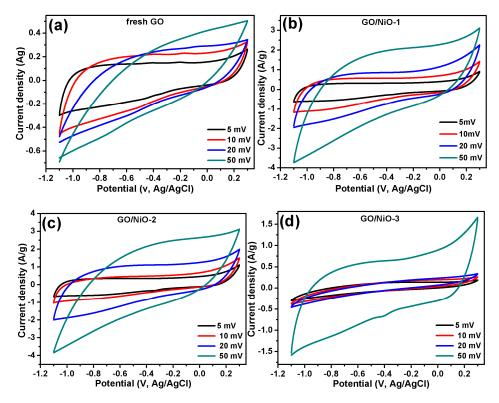
**Figure 12.** CV curves of (a) fresh GO, (b) Ni/GO-1, (c) Ni/GO-2 and (d) Ni/GO with 15 wt% of Ni at scan rates between 5 and 50 mVs<sup>-1</sup>.
