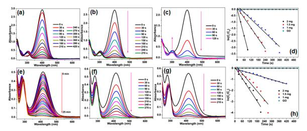
**Figure 10.** UV–vis spectra of the reduction of (**a–c**) 4-NP and (**e–g**) 2-NP in aqueous solution recorded every 30 s using different amount of Ni/GO-1 (1.0, 1.5 and 2 mg). Plots of  $ln[C_t/C_0]$  versus reaction time for the reduction of (**d**) 4-NP and (**h**) 2-NP with NaBH<sub>4</sub> over Ni/GO-1.
