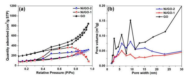
**Figure 8.** (a) Typical N<sub>2</sub> adsorption/desorption isotherm curves of BET isotherm and (b) pore volume of GO, Ni/GO-1 and Ni/GO-2.
