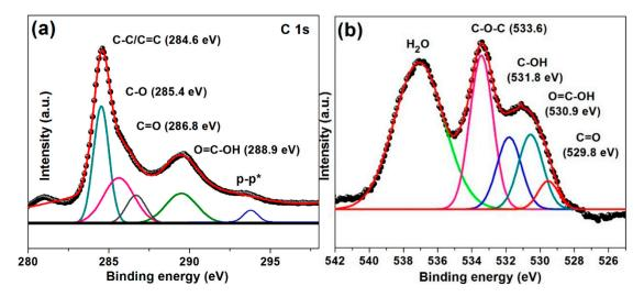
Figure 6. Deconvoluted XPS spectra of (a) C 1s and (b) O 1s peaks of fresh GO.
