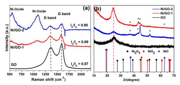
Figure 5. (a) Raman spectra and (b) XRD pattern of GO, Ni/GO-1 and Ni/GO-2.
