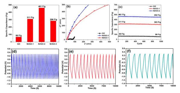
**Figure 13.** (a) Specific capacitance of GO, Ni/GO-1, Ni/GO-2 and Ni/GO-3, (b) Nyquist plots of GO, Ni/GO-1 and Ni/GO-2, (c) cycling stability of GO, Ni/GO-1 and Ni/GO-2, and galvanostatic charge—discharge behavior of (d) GO, (e) Ni/GO-1 and (f) Ni/GO-2.
