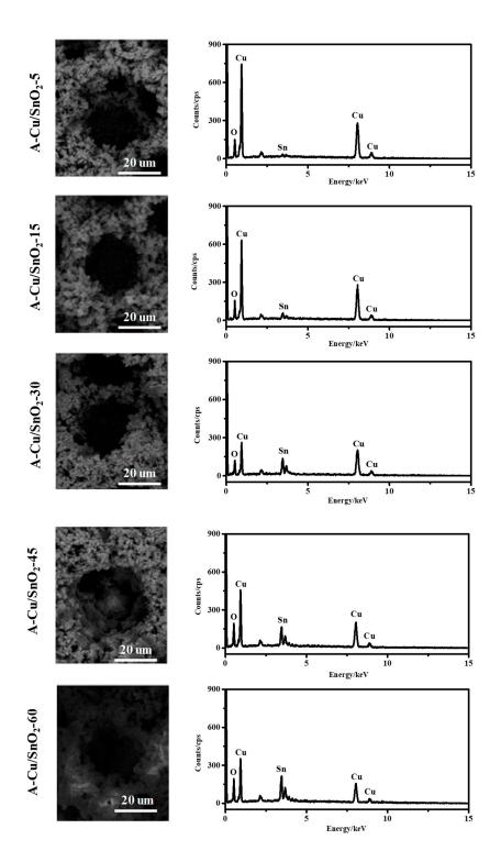
Figure S13. The EDS spectra of A-Cu/SnO<sub>2</sub>-T (T represents the deposition time of SnO<sub>2</sub>).
