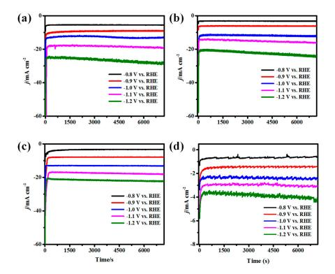
**Figure S7.** The I-t curves during CO<sub>2</sub> electroreduction of (**a**) Cu foam, (**b**) Cu/SnO<sub>2</sub>, (**c**) A-Cu/SnO<sub>2</sub>, (**d**) Sn plate at different voltages in 0.1 M KHCO<sub>3</sub> purged with CO<sub>2</sub> gas.
