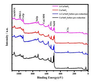
Figure S5. XPS survey spectra of Cu/SnO<sub>2</sub>, A-Cu/SnO<sub>2</sub> before and after pre-reduction.
