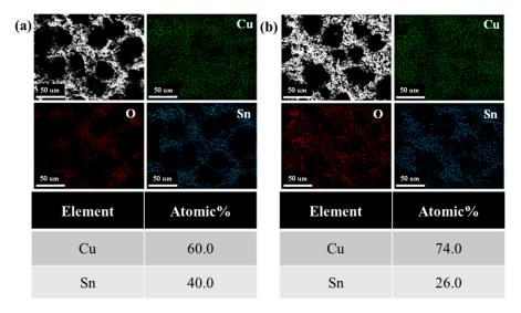
Figure S3. SEM elemental mapping for (a) Cu/SnO<sub>2</sub> and (b) A-Cu/SnO<sub>2</sub> before pre-reduction. The table is EDX analysis identifying.
