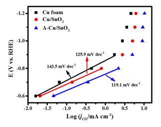
Figure S8. CO partial current density Tafel plots for Cu foam, Cu/SnO2 and A-Cu/SnO2.
