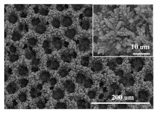
Figure S1. The SEM image of Cu foam.
