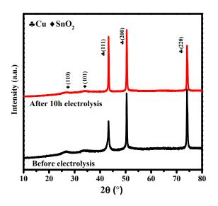
**Figure S14.** XRD patterns of A-Cu/SnO<sub>2</sub> before and after 10 h of CO<sub>2</sub> reduction -1.0 V vs RHE in CO<sub>2</sub>-saturated 0.1 M KHCO<sub>3</sub> solution.
