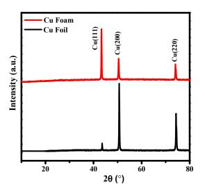
Figure S4. XRD patterns of Cu Foil and Cu foam.
