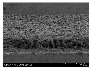
Figure S2. The cross-sectional views of Cu/SnO<sub>2</sub>.
