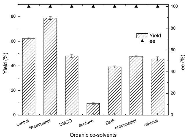
**Figure 3.** Effect of various organic cosolvents on the asymmetric reduction of 4-(trifluoromethyl)acetophenone.
