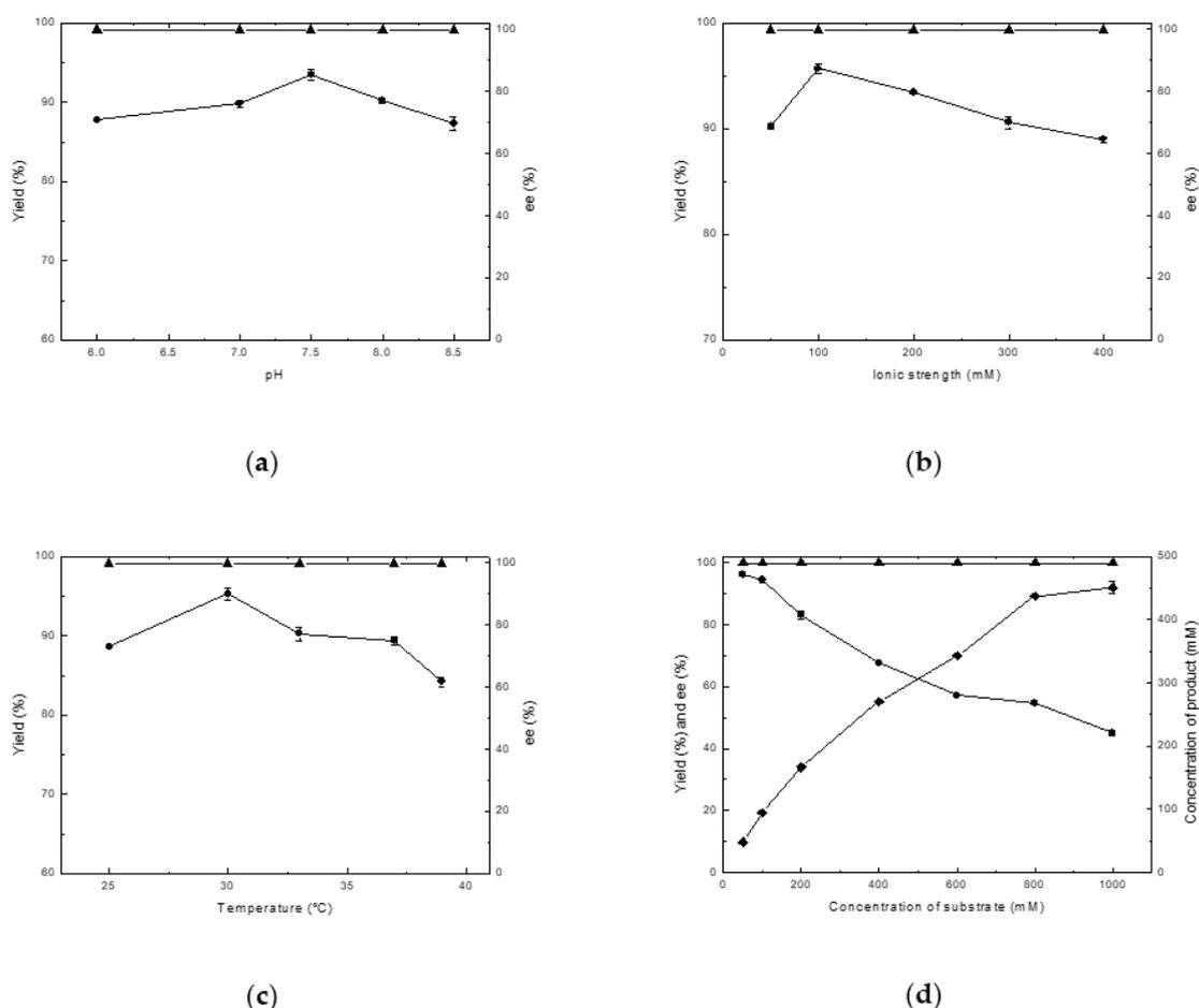
**Figure 5.** Effects of pH. (a) Ionic strength; (b) temperature (c) and substrate concentration (d) on the asymmetric reduction of 4-(trifluoromethyl)acetophenone. Symbols: (●) Yield, (▲) ee and (◆) product concentration.
