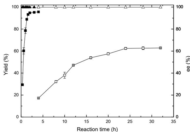
**Figure 6.** Comparison of asymmetric reduction of 4-(trifluoromethyl)acetophenone in isopropanol-buffer medium and aqueous system. Symbols: (■) Yield in 15% (v/v) isopropanol-buffer solution and (□) yield in buffer solution, (▲) ee in 15% (v/v) isopropanol-buffer solution and (△) ee in buffer solution.
