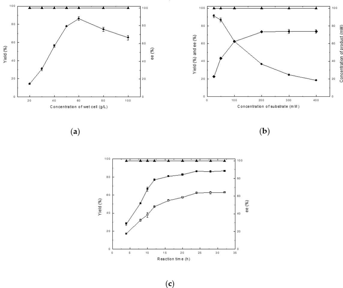
**Figure 2.** Effects of cell concentration. (a) Substrate concentration; (b) reaction time (c) on the asymmetric reduction of 4-(trifluoromethyl)acetophenone in phosphate buffer. Symbols: (●) Yield and (▲) ee; (◆) product concentration; (■) yield at 50 mM 4-(trifluoromethyl)acetophenone and (□) yield at 100 mM 4-(trifluoromethyl)acetophenone.
