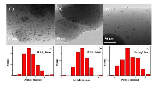
Figure S1. TEM images and corresponding size distribution of  $Pt_{0.8}/SiO_2$ -Shiff (a),  $Pt_{0.5}/SiO_2$ -Shiff (b) and  $Pt_{0.3}/SiO_2$ -Shiff (c).
