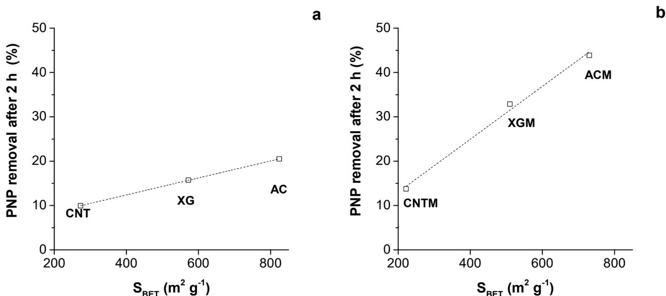
**Figure S1.** Correlation between specific surface area and the PNP removal after 2 h of adsorption with the carbon supports undoped (a) and N-doped with melamine (b) (pH= 3.0, T= 30 °C, [support] = 0.25 g L<sup>-1</sup> and [PNP] = 3.6 mmol L<sup>-1</sup>).
