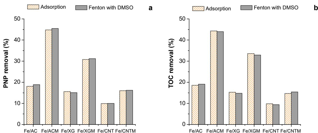
**Figure S2.** PNP (a) and TOC (b) removal after 2 h of adsorption or Fenton's oxidation in presence of DMSO with the catalysts (pH= 3.0, T= 30 °C, [catalyst] = 0.25 g L<sup>-1</sup>, [H<sub>2</sub>O<sub>2</sub>]<sub>when used</sub> = 29 mmol L<sup>-1</sup>, [PNP] = 3.6 mmol L<sup>-1</sup> and H<sub>2</sub>O<sub>2</sub>:PNP molar ratio = 8.1, when H<sub>2</sub>O<sub>2</sub> was used).
