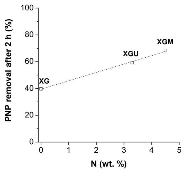
**Figure S3.** Relationship between PNP removal after 2 h of Fenton reaction and N-amount of N-doped xerogels (pH= 3.0, T= 30 °C, [support] = 0.25 g L<sup>-1</sup>, [H<sub>2</sub>O<sub>2</sub>] = 29 mmol L<sup>-1</sup>, [PNP] = 3.6 mmol L<sup>-1</sup> and H<sub>2</sub>O<sub>2</sub>:PNP molar ratio = 8.1).
